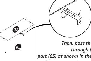
Then, pass the hardware (J) through the hole of the part (05) as shown in the figure above. You will need a pencil to mark where you should drill the wall with a 3/8" drill bit to put in the hardware (I).
