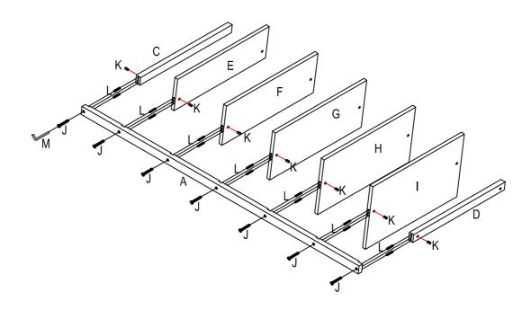
Attach Nut (K) to Top Cross Bar (C), Bottom Cross Bar (D), Top Panel (E), Shelf (F), (G), (H), Bottom Panel (I). Then attach Rsf Rail (B) to Top Cross Bar (C), Bottom Cross Bar (D) and Top Panel (E), Shelf (F), (G), (H), Bottom Panel (I) by using Wood Dowel (L) and Bolt (J) with Allen Key (M).
