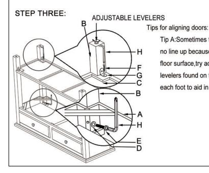
Tip A:Sometimes the doors will no line up because of an uneven floor surface, try adjusting the levelers found on the botton of each foot to aid in correcting.
