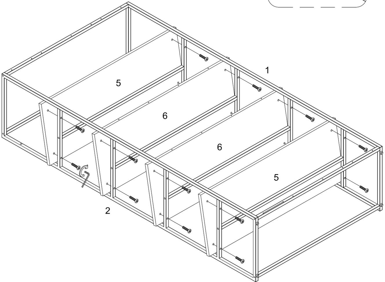
Attach part (5, 6) to part (1, 2) using bolt (A) with hex key (D) per diagram.
