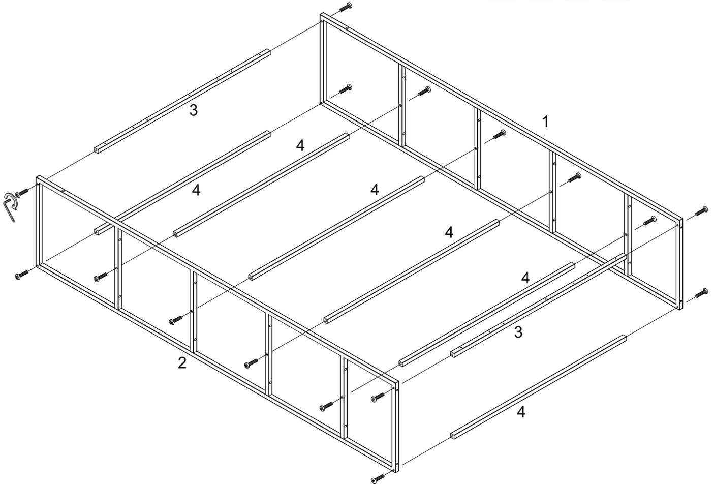
Attach part (3, 4) to part (1, 2) using bolt (A) with hex key (D).
