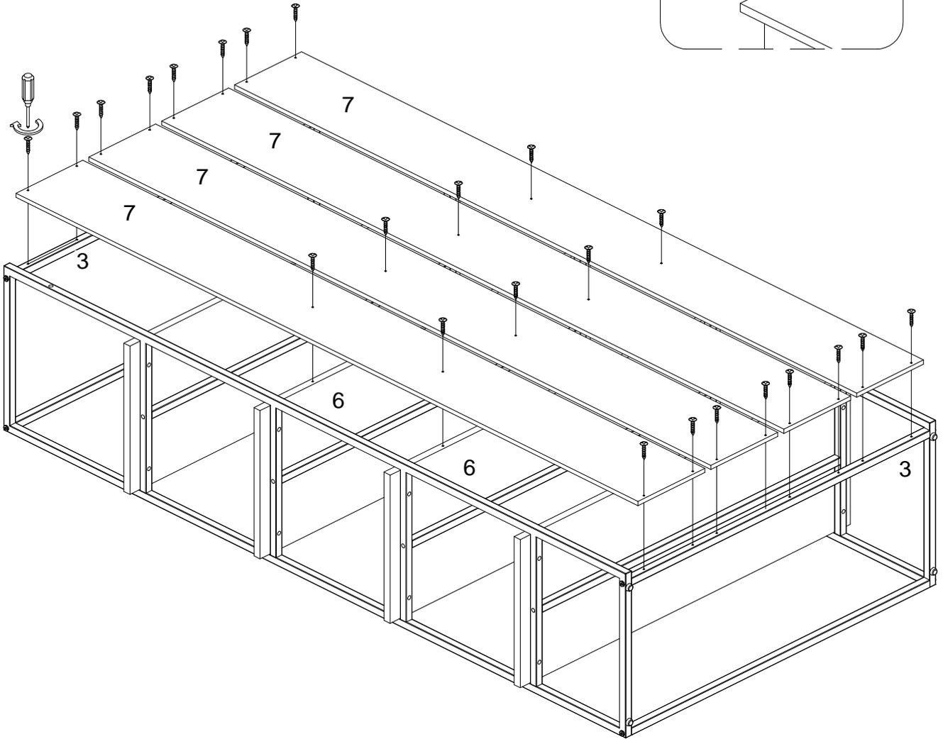
Attach part (7) to part (3, 6) using screw (B) with Philips head screwdriver.
