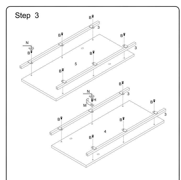
Using bolt (B) attach part (3) to parts (4,5) ,then using bolt (H) attach bracket (M) into part (3) with hex key (N) as per diagram.
