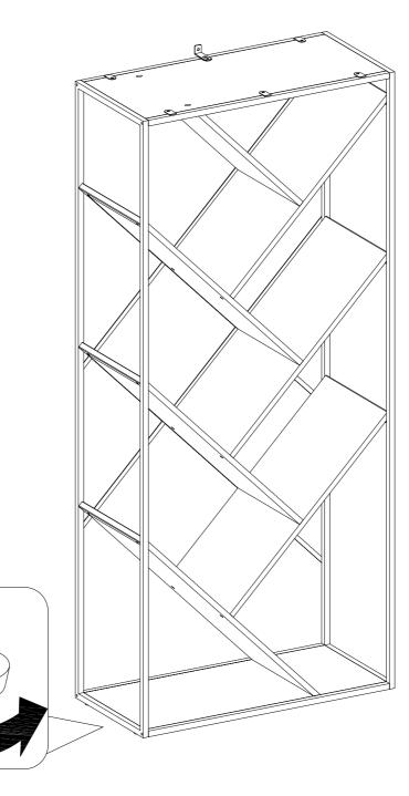
If necessary, adjust the pre-attached Floor Levelers at the bottom of metal legs to level the unit.
