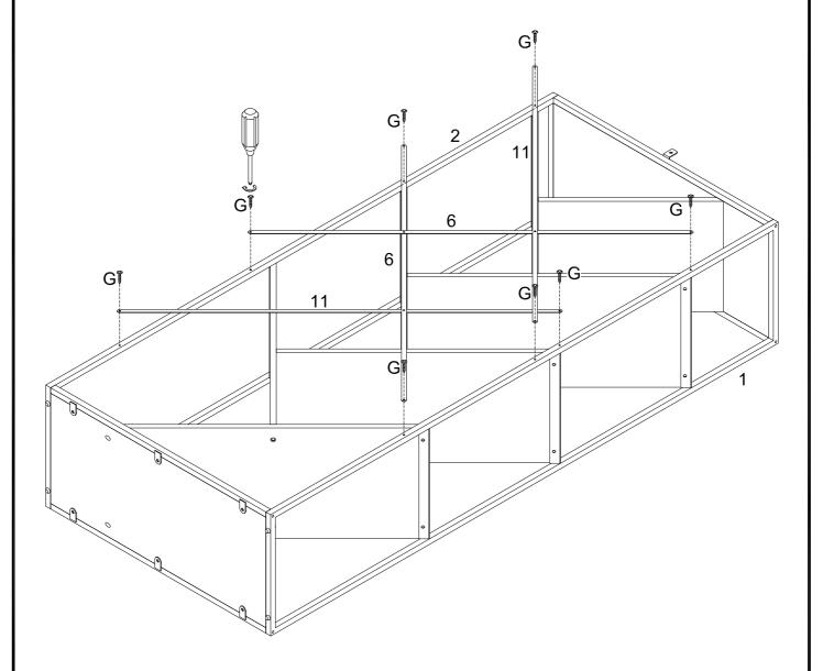
Using screw (G) attach parts (6,11) into parts (1,2) with Philips head screwdriver as per diagram.
