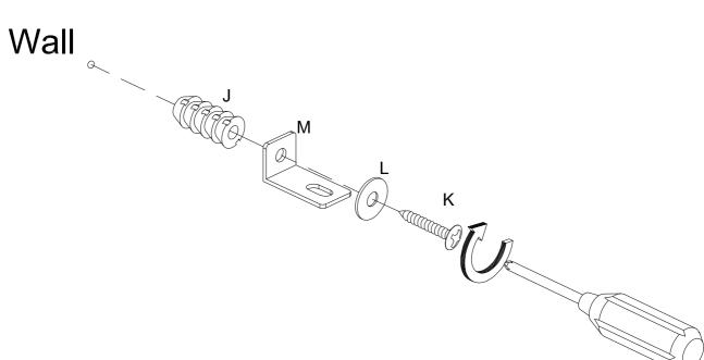
Using screw (K) attach Flat washer (L) to bracket (M) to Wall anchor (J) to wall with Philips head screwdriver as per diagram.
