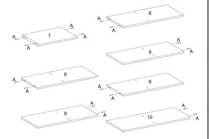
Insert wooden dowel (A) into parts (7,8,9,10) as per diagram.
