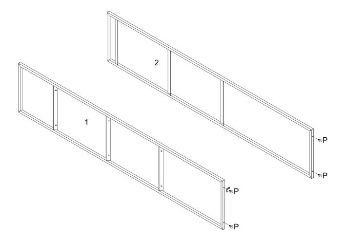
Secure feet (P) at the bottom of parts (1,2) as per diagram.
