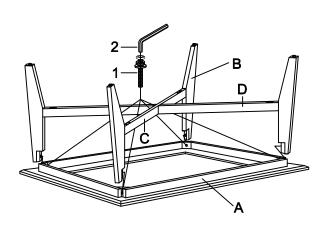
This step needs installation of four Bolts (#1).
