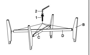
This step needs installation of four Bolts (#1).
