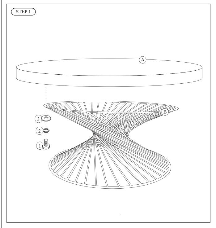
Attach Top (A) to Base (B) using 4 Allen Bolts (1), 4 Spring Washers (2), and 4 Flat Washers (3). Tighten all bolts using Allen Wrench (4) provided. The assembly is now complete.
