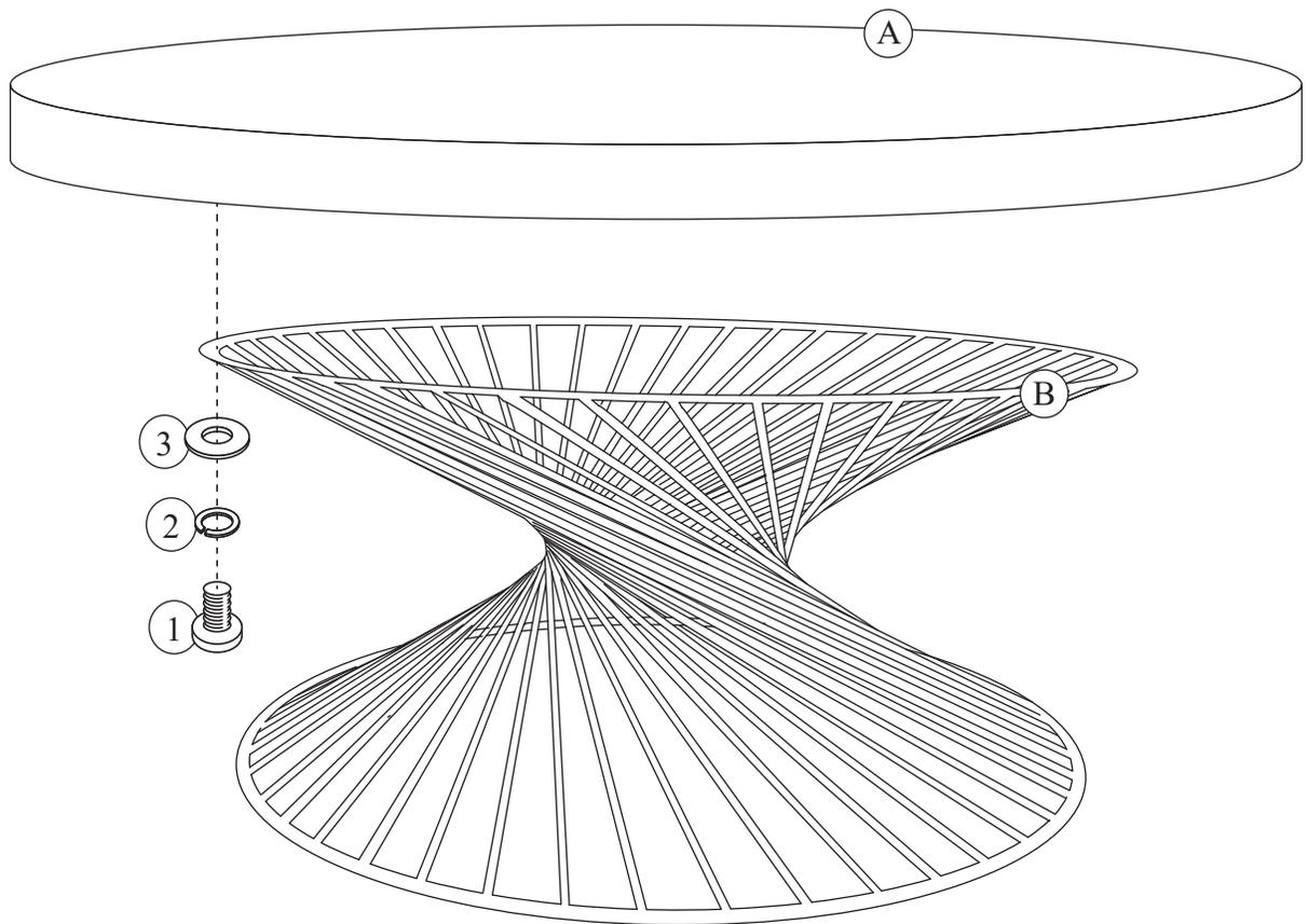
Attach Top (A) to Base (B) using 4 Allen Bolts (1), 4 Spring Washers (2), and 4 Flat Washers (3). Tighten all bolts using Allen Wrench (4) provided. The assembly is now complete.
