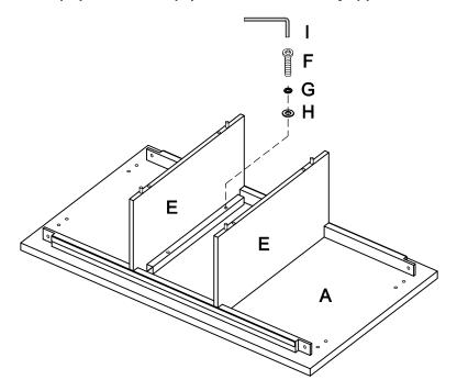
Attach Bottom Panel (C) to the Vertical Panel (E) by using Flat Washer (H), Lock Washer (G), Bolt (F) with L-Allen Key (I) as below showing.
