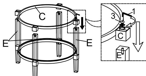
Step 4: Using Antiskid Pad (4) and Metal Cap (F) to the Top frame (C)
