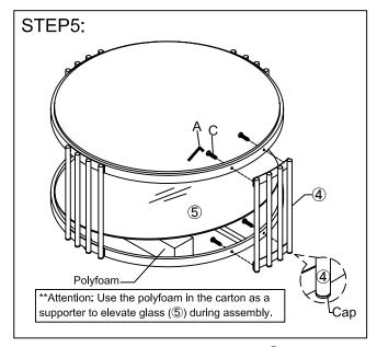
Assembly the last side frame (4) to the assembled table with bolts (C) by use of Allen key (A).
