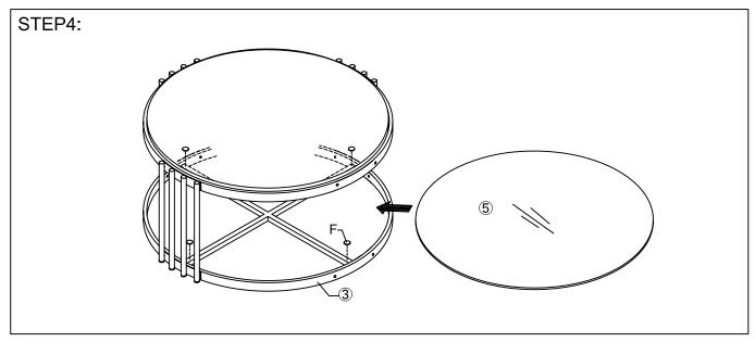
Stick rubber mats (F) onto bottom frame (③), then, place the glass (⑤) onto the assembled table.
