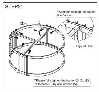
Assembly bottom frame (③) to side frames (④) with bolt (C) by use of Allen key (A).
