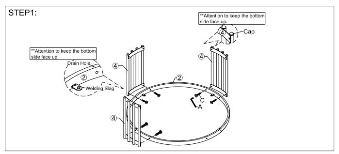
Assembly three side frames (4) to the top frame (2) with bolt (C) by use of Allen key (A).
