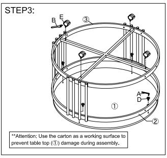
Assembly top frame (2) to table top (1) with bolts (D) by use of Allen key (A). Then screw wheels (E) onto the bottom frame (3) by using the wrench (B).
