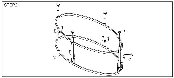
Assembly top frame (②) to leg tubes (④) with bolts (C) by use of Allen key (A). Then screw the levelers (D) into the threaded holes on leg tubes (④).
