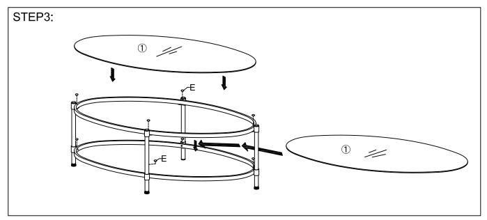
Stick rubber mats (E) onto top frame (②) & bottom frame (③), then, place the glass (①) onto the assembled table.
