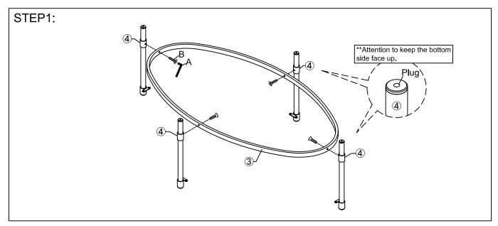
Assembly leg tubes (4) to the bottom frame (3) with bolts (B) by use of Allen key (A).
