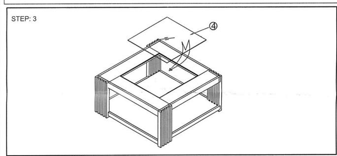
Turn table to its feet . Put glass in top frame. Assembly completely
