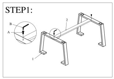
Lay the metal frames upside down, on a carpeted or protective surface, to avoid damage. Attach the stretch between the two frames by using the provided screws
