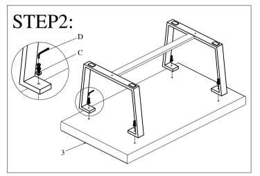
Lay the table top upside down, on a carpeted or protective surface, to avoid damage. Attach the legs, using the provided screws and washers, aligning the holes, into the threaded inserts, tighten securely.
