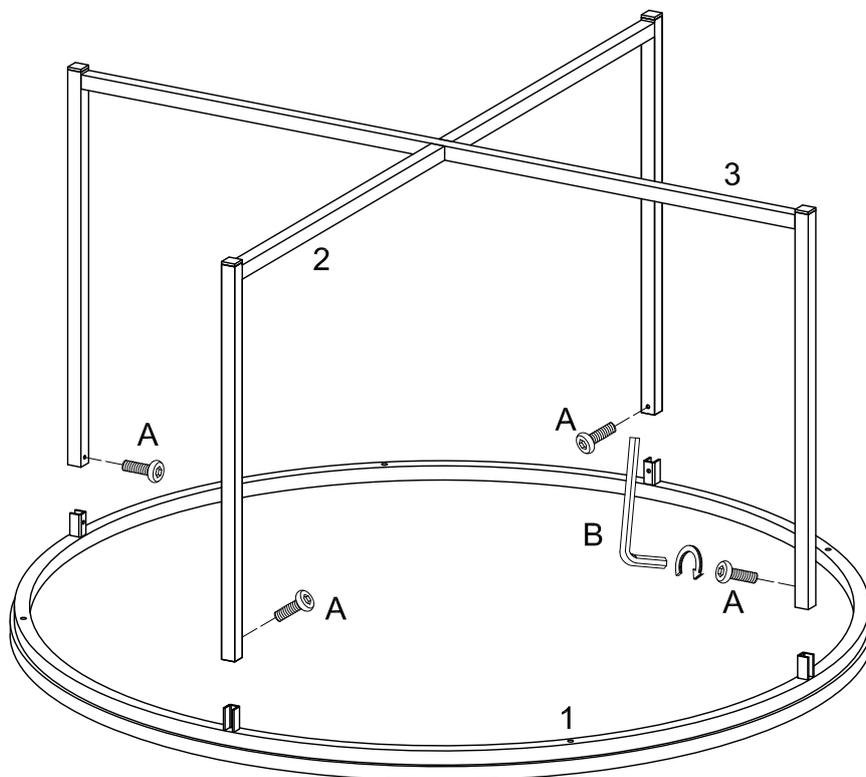
Use wrench (B), to secure legs (2,3) to table top (1) with bolts (A).
