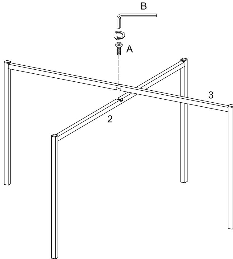
Use wrench (B), to secure legs (2,3) with bolt (A).
