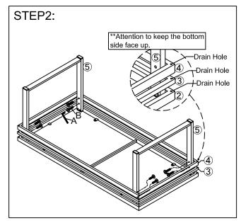
Assembly 2nd frame (③) & 3rd frame (④) to side frames (⑤) with bolt (B) by use of Allen key (A).
