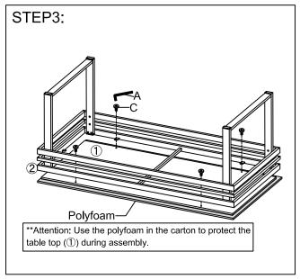
Assembly top frame (2) to table top (1) with bolt (C) by use of Allen key (A).
