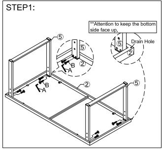
Assembly side frames (5) to top frame (2) with bolt (B) by use of Allen key (A).
