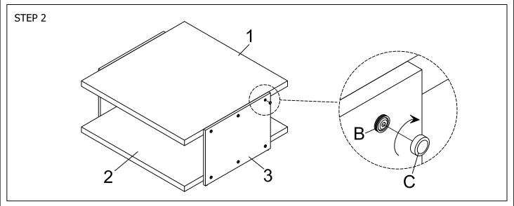
Assemble the metal caps (C) to the Allen bolts on the Arcrylic Side panel (3)
