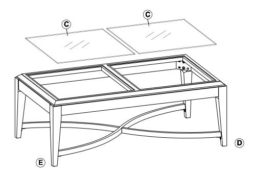
Turn the assembly table in step 1 up right side then insert the Glass (C) into the Table Top (A).
