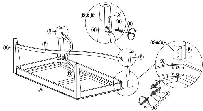
Place the Table Frame (A) upside down on the soft surface to prevent finish from scratching. Attach the Right (D), Left (E) Legs to the holes at the corners of the Table Frame (A), secure Long Bolt (1), Lock Washer (2), Flat Washer (3), with Allen Key (6). Assemble the X Stretcher (B) to the Right (D), Left (E) Legs by using Bracket (4), Short Bolt (5), tighten with Allen Key (6). Fully tighten all bolts at this step.
