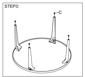
Insert foot nail (C) into the hole on leg as shown in illustration.
