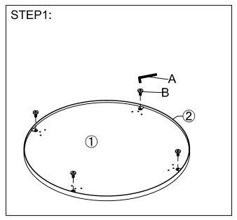
Assembly table top (1) to top frame (2) with bolt (B) by use of Allen key (A).
