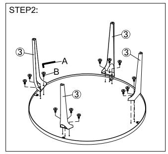
Assembly legs ( $\mathfrak{J}$ ) to table top ( $\mathfrak{I}$ ) with bolt (B) by use of Allen key (A).
