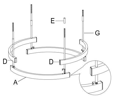
Attach Connector Tubes (E) to each Long Bolt (G) and follow with Stretchers (B) as shown. Repeat step to add another level of Stretchers (B).
