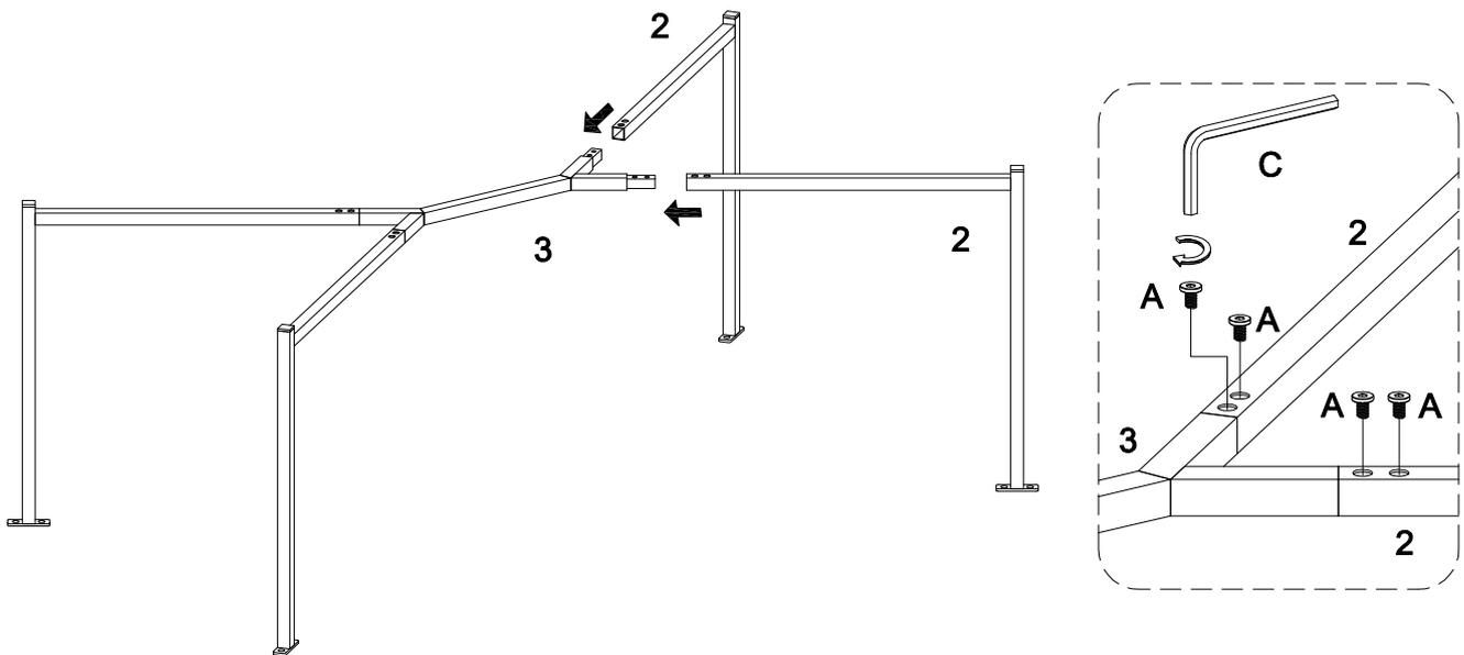
Insert part (3) into legs (2), then use wrench (C) to secure them with bolt (A).
