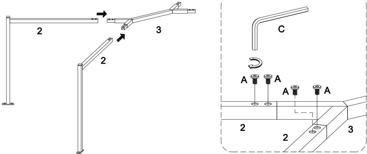
Insert part (3) into legs (2), then use wrench (C) to secure them with bolt (A).
