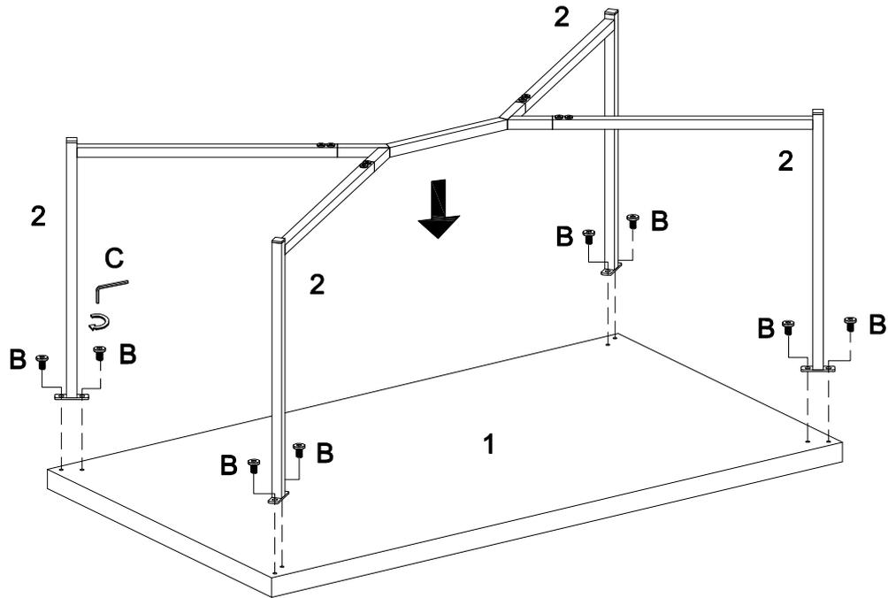
Use wrench (C) to secure legs (2) to top panel (1) with bolt (B).
