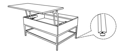
Tip B: Sometimes product will not line up because of an uneven surface the furniture rests on. In that case try adjusting the levelers found on the bottom of each leg to aid in correcting.
