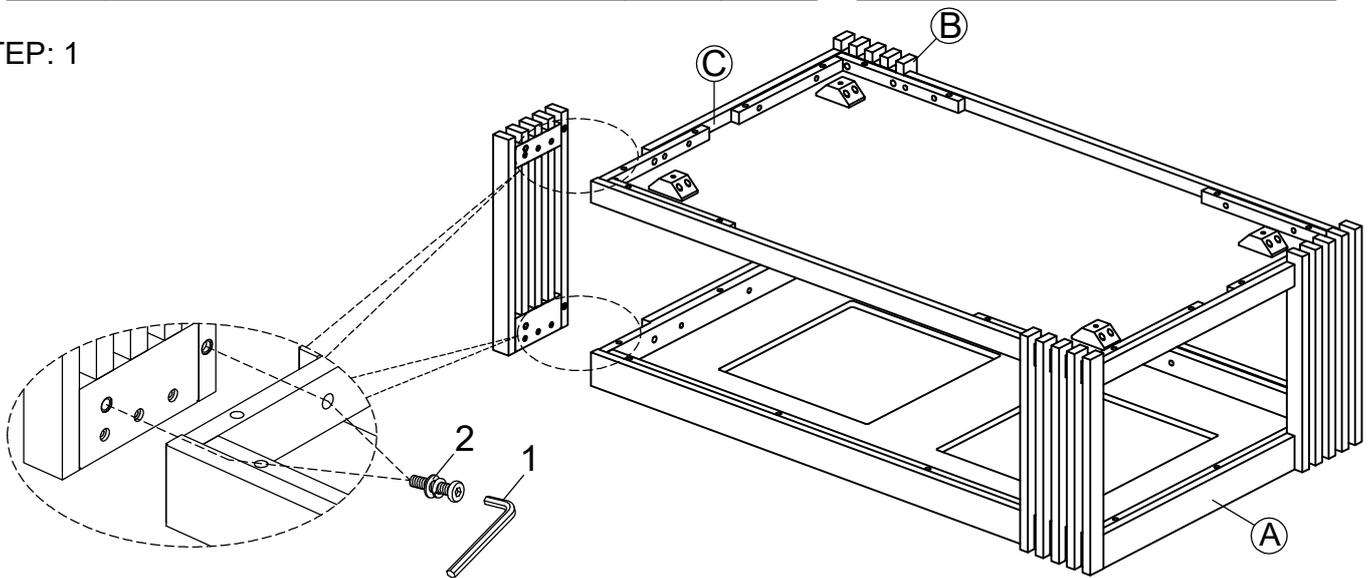
Caution : first step do not tighten the bolts, after turn up all the tables & put it on flat surface ,then can tighten all bolts by using Allen Key.
