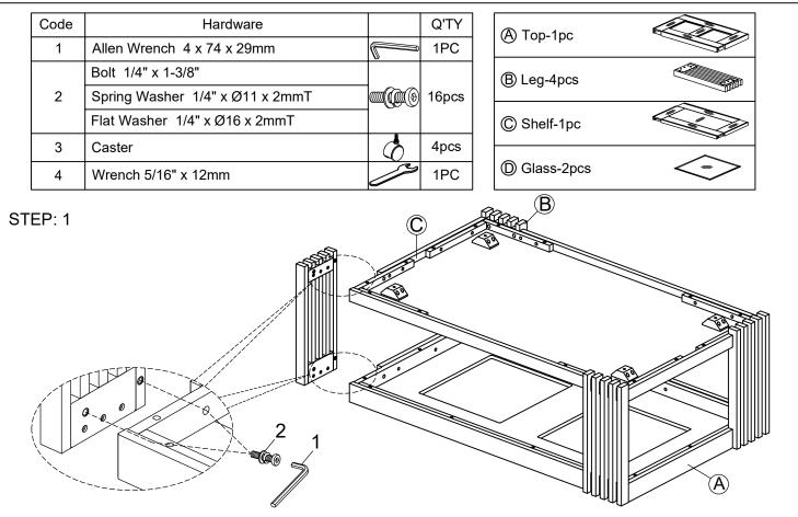
Caution : first step do not tighten the bolts, after turn up all the tables & put it on flat surface ,then can tighten all bolts by using Allen Key.
