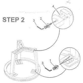
2.Attach Table bottom to the leg by using bolt, flat washer, spring washer(2) and allen wrench(3). Then attach the third leg to the back of the table top by using bolt, flat washer, spring washer(1) and allen wrench(3). Last, assemble the third leg to table bottom by using bolt, flat washer, spring washer(2) and allen wrench(3).
