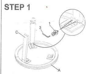
1. Put the table top face down on a smooth soft surface to prevent damage. Only attach 2 Table legs to the back of the table top by using flat washer, spring washer, bolt(1) and allen wrench(3).
