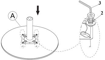
**STEP 3** Assemble the Bottom round table by bolt (1) and tighten with Allen key (3).
