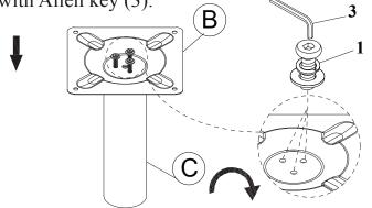
**STEP 2** Assemble the STEP 1 to the Top table (A) by bolt (2) and tighten with Allen key (3).
