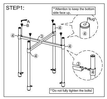
Assembly leg tubes (4) to the bottom frame (3) with bolts (B) by use of Allen key (A).
