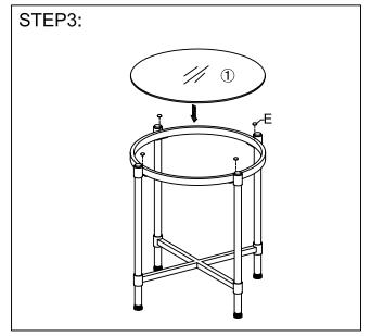
Stick rubber mats (E) onto top frame ((2)), then, place the glass ((1)) onto the assembled table.
