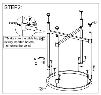
Assembly top frame (②) to leg tubes (④) with bolts (C) by use of Allen key (A). Then screw the levelers (D) into the threaded holes on leg tubes (④).
