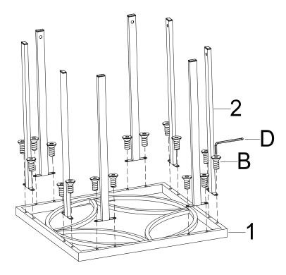
Step 2) Attach metal bottom frame (#3) to metal legs (#2) by using bolt (A) as shown then tighten all bolts firmly.
