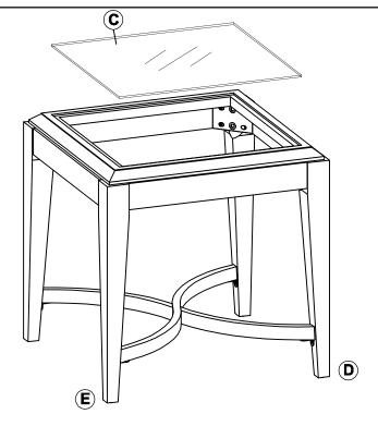
Turn the assembly table in step 1 up right side then insert the Glass (C) into the Table Top (A).
