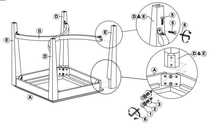
Place the Table Frame (A) upside down on the soft surface to prevent finish from scratching. Attach the Right (D), Left (E) Legs to the holes at the corner of the Table Top (A), secure Long Bolt (1), Lock Washer (2), Flat Washer (3), with Allen Key (6). Assemble the X Stretcher (B) to the Right (D), Left (E) Legs by using Bracket (4), Short Bolt (5), tighten with Allen Key (6). Fully tighten all botls at this step.
