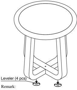
Leveler are pre-installed on the Table leg.
