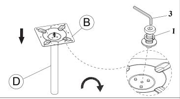
**STEP 3** Assemble the Bottom round table by bolt (1) and tighten with Allen key (3).
