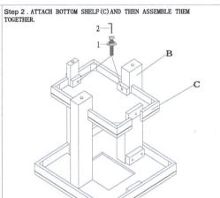
This step needs installation of three bolts(1) .
