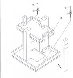
This step needs installation of two bolts(1).
