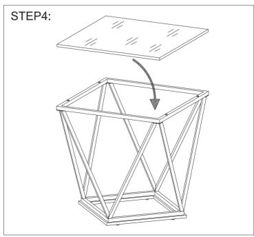
Turn base upright and insert insert the glass tips into the upper frame
