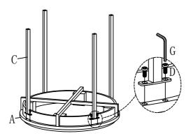
Attach Bottom Frame (B) to Support Rod (C) using, Bolt (E), Flat Washer (F) with Allen Key (G).
