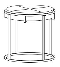
This page lists all the contents included in the box. Please take the time to identify the hardware as well as the individual components to this product. As you unpack and prepare for assembly, place the contents on a carpeted or padded area to protect them from damage. Attach Support Rod (C) to Top Panel (A) using Bolt (D) with Allen Key (G).
