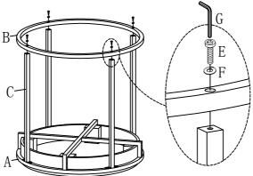
Adjust the Pre-installed Levelers at the Bottom Frame (B) until the End Table is level with the ground.
