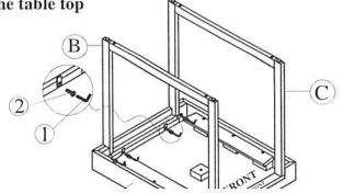
STEP 2: Assemble the leg frame front, leg frame back with 2 stretchers
