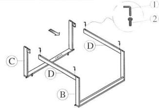
STEP 4: Pull the drawer back and assemble the bolt.
