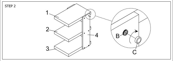
Assemble the metal caps (C) to the Allen bolts on the Arcrylic Side panel (4)
