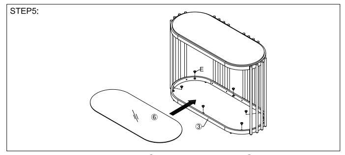
Insert suckers (E) onto bottom frame (③), then, place the glass (⑥) onto the assembled table.
