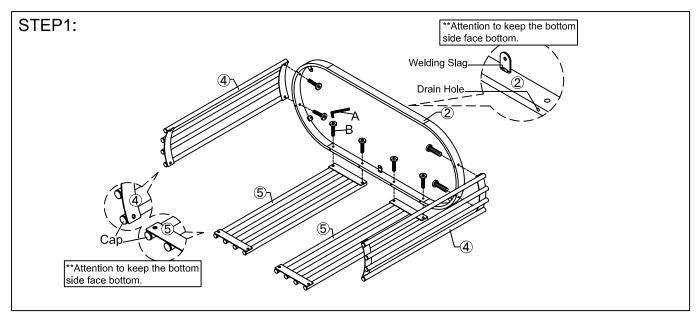
Assembly side frames (4 & 5) to the top frame (2) with bolts (B) by use of Allen key (A).
