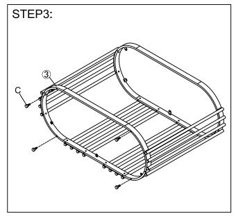
Screw the levelers (C) into the threaded holes on bottom frame (3).
