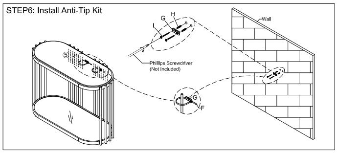
Mark the location on the wall for mounting plastic bracket (G). Drill a 3/8 inch hole in the wall and insert anchor (H). Secure the bracket (G) to the wall using the screw (I). Place the table so the back side of unit is lined with the bracket (G) on the wall, then lace an end of the strap (F) down through the tube of the side frames (⑤) and the bracket (G) on the wall.
