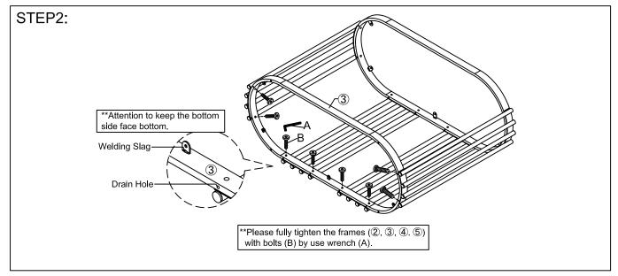
Assembly bottom frame (3) to side frames (4 & 5) with bolts (B) by use of Allen key (A).
