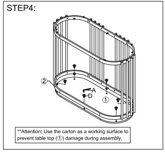
Assembly top frame (2) to table top (1) with bolts (D) by use of Allen key (A).
