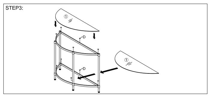
Stick rubber mats (D) onto table frame (2), then, place the glass (1) onto the assembled table.
