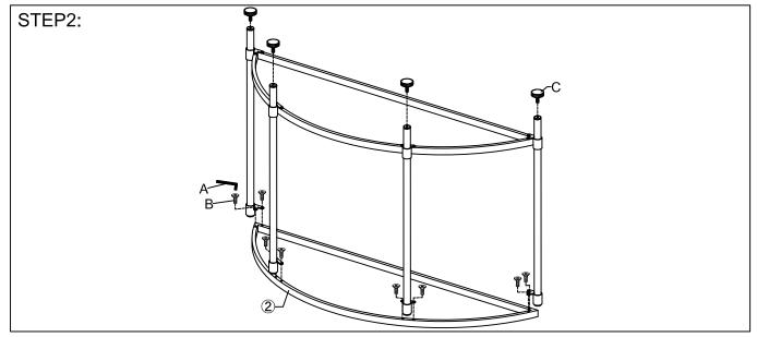
Assembly another table frame (2) to leg tubes (3, 4, 5) with bolts (B) by use of Allen key (A). Then screw the levelers (C) into the threaded holes on leg tubes (3, 4, 5).
