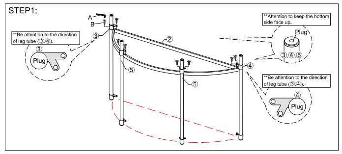
Assembly leg tubes (3, 4, 5) to a table frame (2) with bolts (B) by use of Allen key (A).
