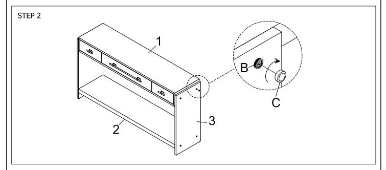
Assemble the metal caps (C) to the Allen bolts on the Arcrylic Side panel (3)
