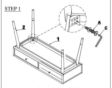
Note: do not tighten all the bolts and screws until the final assembling steps.
