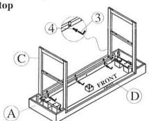
STEP 3: Pull the drawer back and assemble the bolt.
