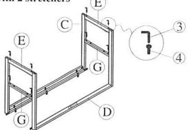
STEP 2: Attach the legs frame to the table top. Note: Attach the leg frame front same side with the table top
