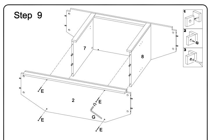
Secure part (2) to frame assembly using bolts (E) as shown in the diagram.
