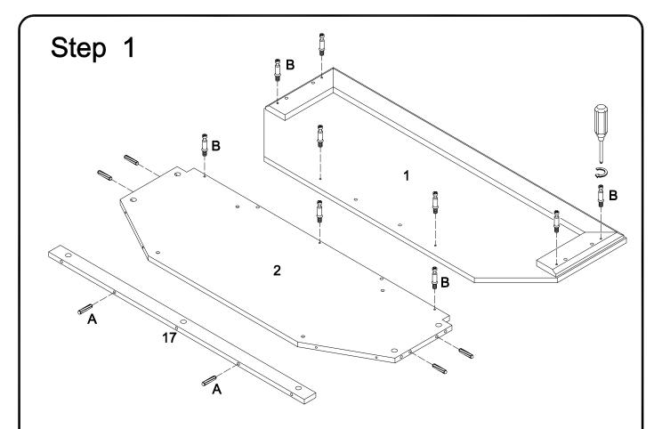
Attach cam bolts (B) to parts (1) and (2). Insert wooden dowels (A) into parts (2) and (17).
