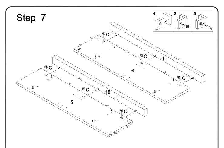
Attach cam locks (C) to parts (11,18) to connect to part (5,6) as shown in the diagram.
