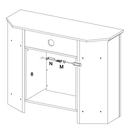
Be sure the fire place insert is positioned all the way forward in place. Use screw (M) to secure the L-shape bracket (N) to the side panels (8). Position the adjustable L-bracket to hold the Fireplace insert in place.
