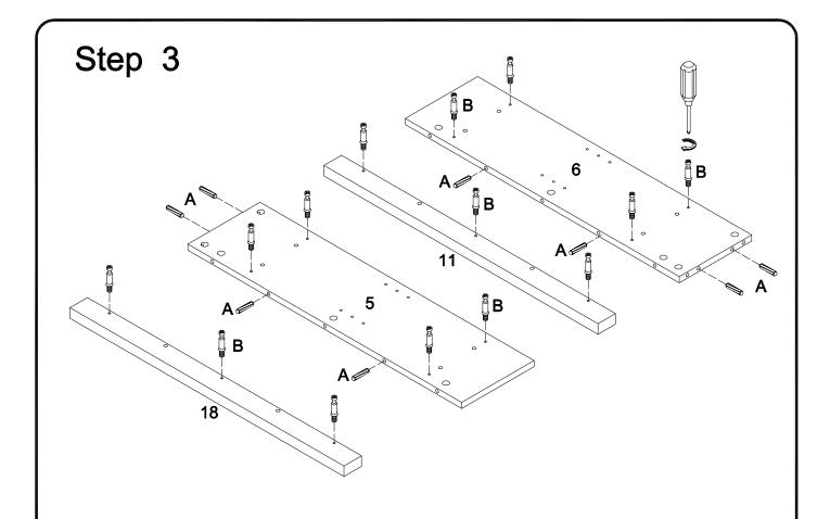
Attach cam bolts (B) to parts (5,6) and (11,18). Insert wooden dowels (A) into parts (5) and (6).
