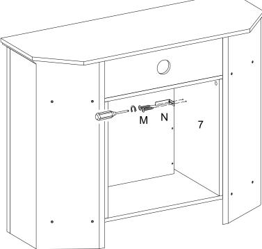
Be sure the fire place insert is positioned all the way forward in place. Use screw (M) to secure the L-shape bracket (N) to the side panels (7). Position the adjustable L-bracket to hold the Fireplace insert in place.
