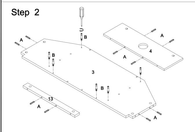
Attach cam bolts (B) to part (3). Insert wooden dowels (A) into parts (3,4) and (13).
