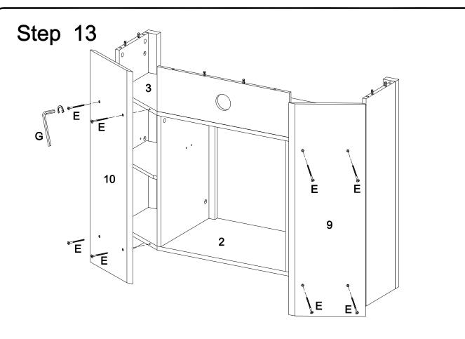
Attach parts (9) and (10) to frame assembly using bolts (E) as shown in the diagram.
