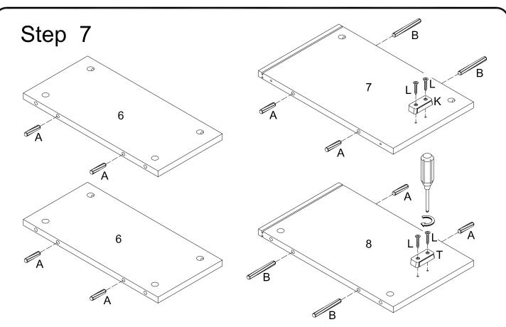
Insert wooden dowels (A, B) into panels (6, 7, 8) as shown in the diagram. Secure left door stopper (K) to panel (7) using screws (L). Secure right door stopper (T) to panel (8) using screws (L).
