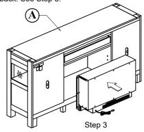
Step 2: On the back, pull the console back panel to install the Firebox. See Step 2.
