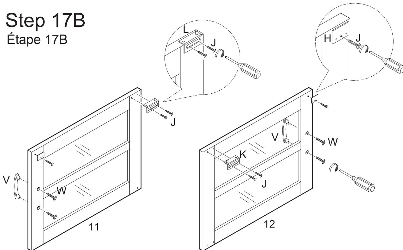
Attach handles (V) to doors (11, 12) using handle bolts (W). Attach door stopper plates (H) to doors (11, 12) using screws (J). Attach door hinge (L) to door (11) using screws (J). Attach door hinge (K) to door (12) using screws (J).
