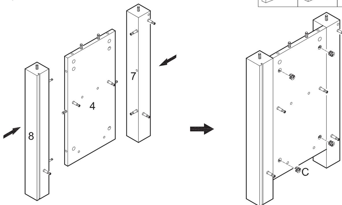
Attach legs (7,8) to panel (4) using cam bolts and dowels as guides. Insert cam locks (C) into panel (4) and tighten with a screwdriver.
