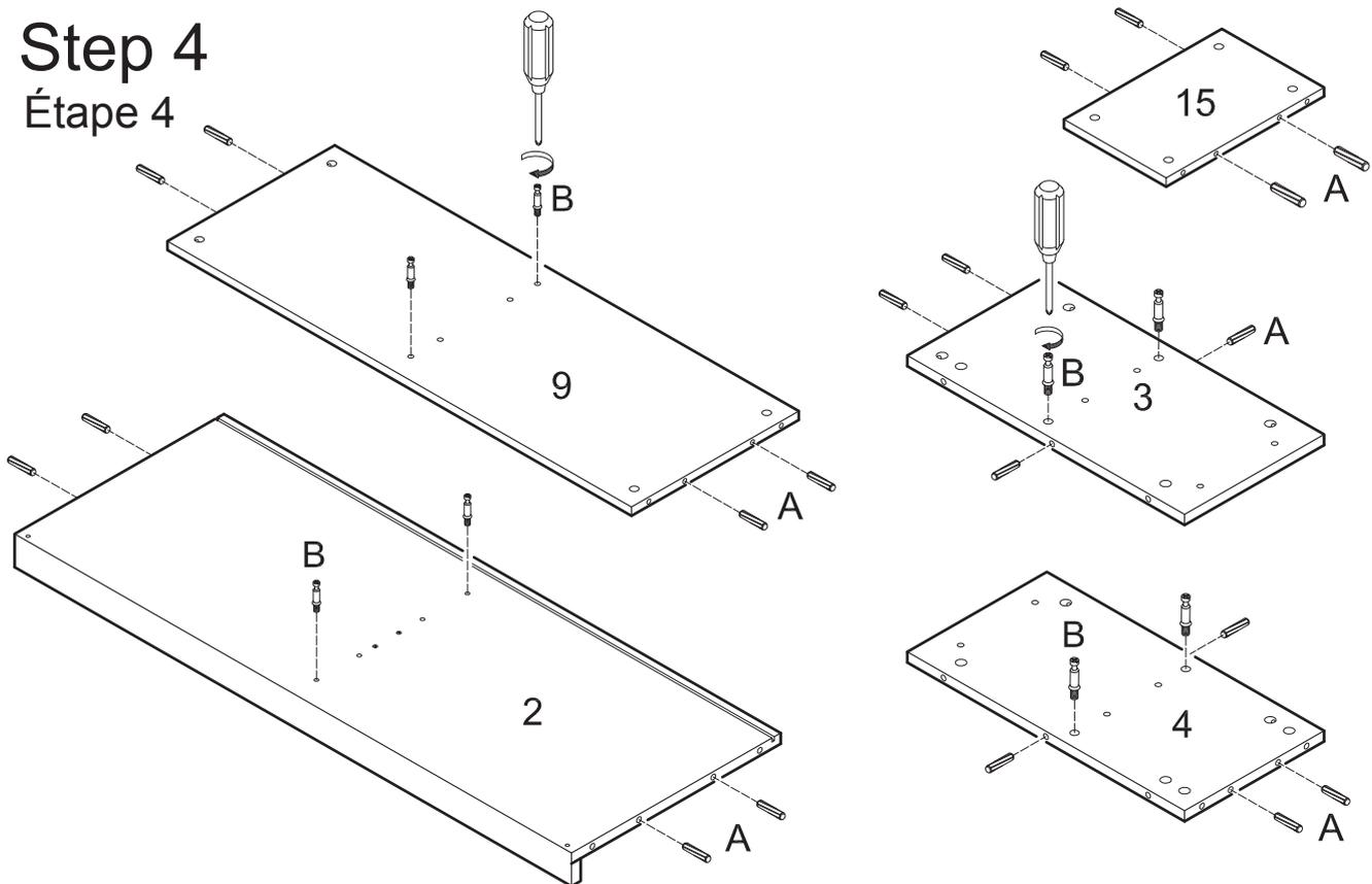
Insert dowels (A) into panels (2,3,4,15) and shelf (9). Screw cam bolts (B) into panels (2,3,4) and shelf (9).
