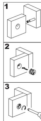
Insert cam locks (C) into the frame assembly. Attach stand top (1) to the frame assembly using cam bolts and dowels as guides. Tighten cam locks (C) with a screwdriver.
