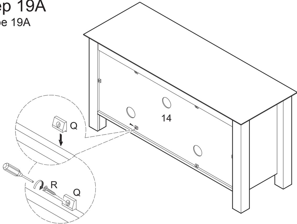
Secure back panel (14) using plastic wedges (Q) and screws (R).
