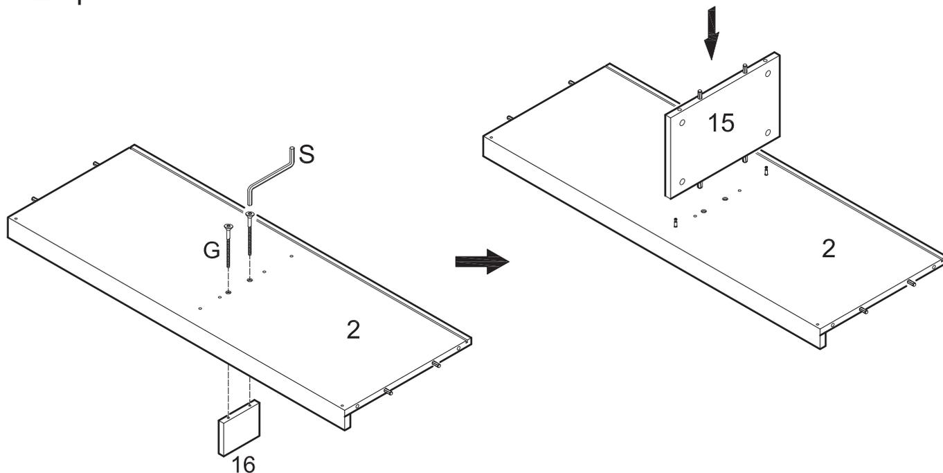
Attach support leg (16) to panel (2) using long bolts (G). Tighten long bolts (G) with wrench (S). Attach panel (15) to panel (2) using cam bolts and dowels as guides.
