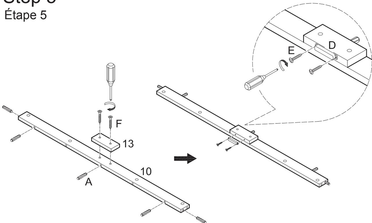
Insert dowels (A) into slat (10). Attach block (13) to slat (10) using screws (F). Attach door stopper (D) to block (13) using screws (E).
