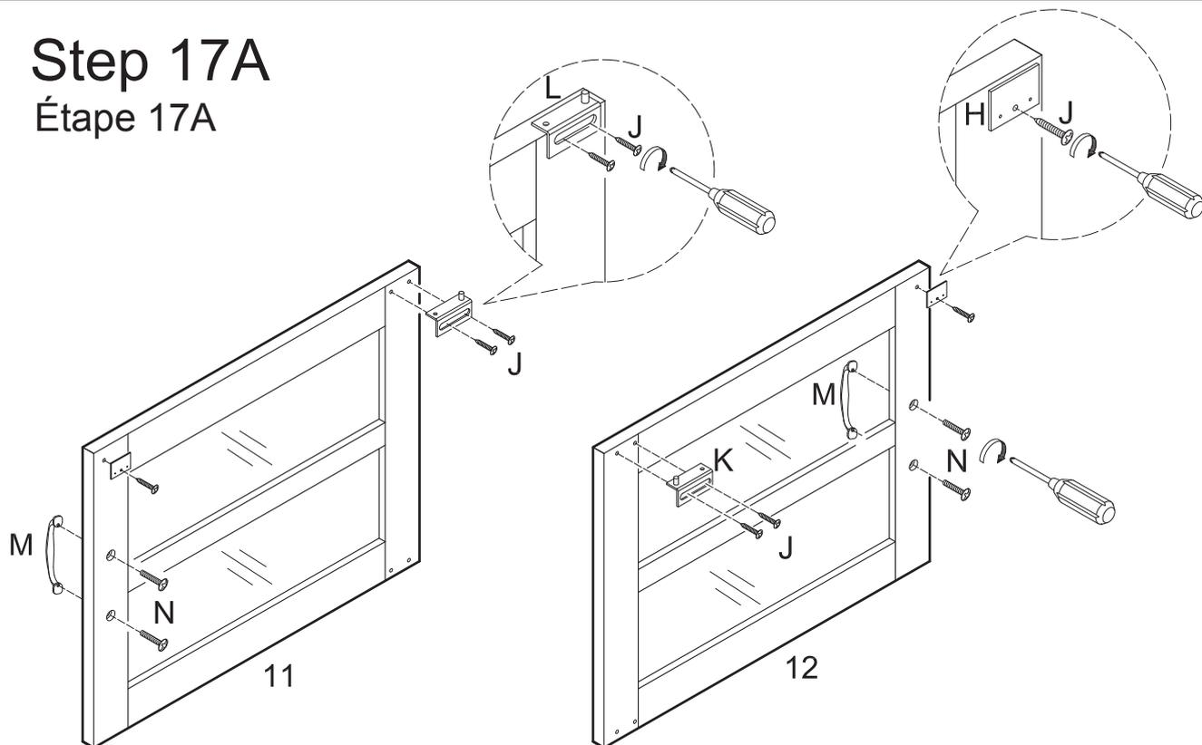
Attach handles (M) to doors (11, 12) using handle bolts (N). Attach door stopper plates (H) to doors (11, 12) using screws (J). Attach door hinge (L) to door (11) using screws (J). Attach door hinge (K) to door (12) using screws (J).
