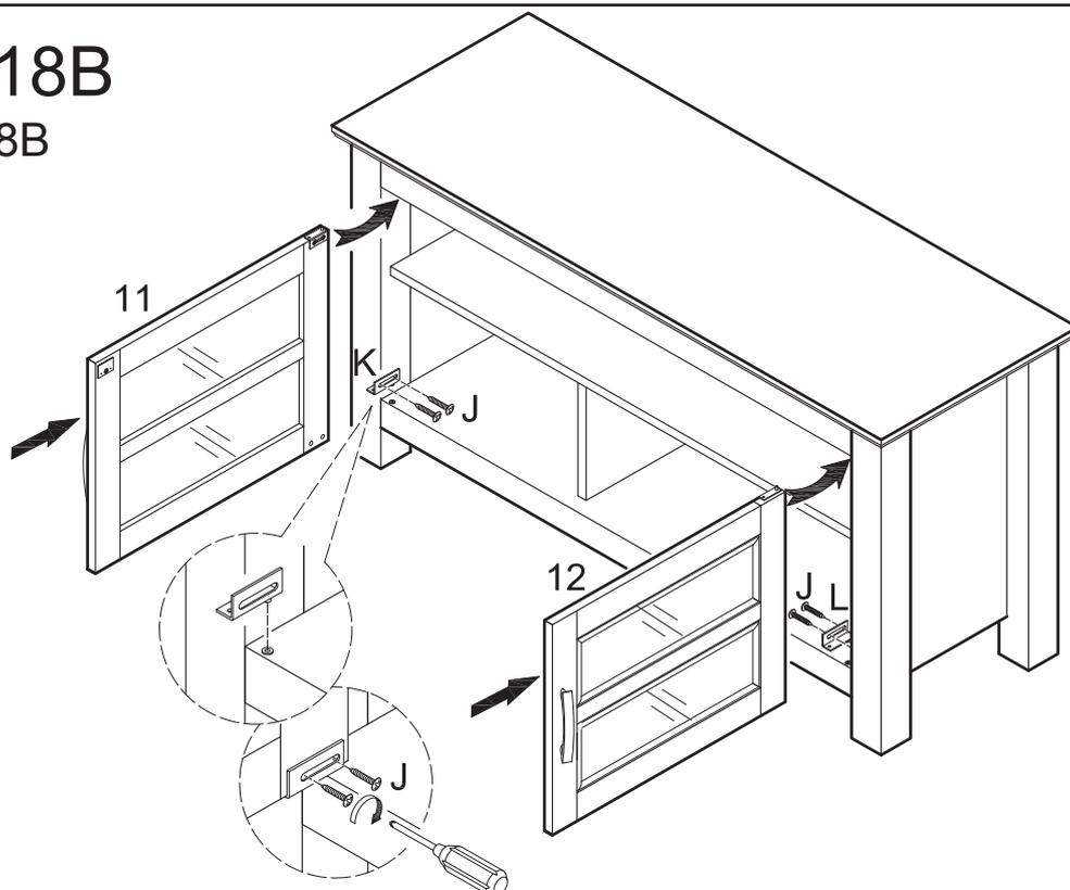
Insert door hinge (K) into left bottom plastic pivot (P). Slide door (11) into place. Attach door hinge (K) to door (11) using screws (J). Insert door hinge (L) into right bottom plastic pivot (P). Slide door (12) into place. Attach door hinge (L) to door (12) using screws (J).
