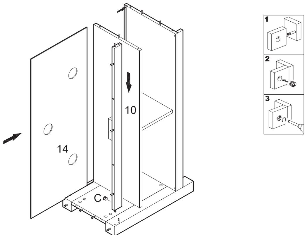
Attach slat (10) to the assembly from the previous step using cam bolt and dowel as guides. Insert cam lock (C) into slat (10) and tighten with a screwdriver. Slide back panel (14) into place along the grooves at the back of the frame assembly.
