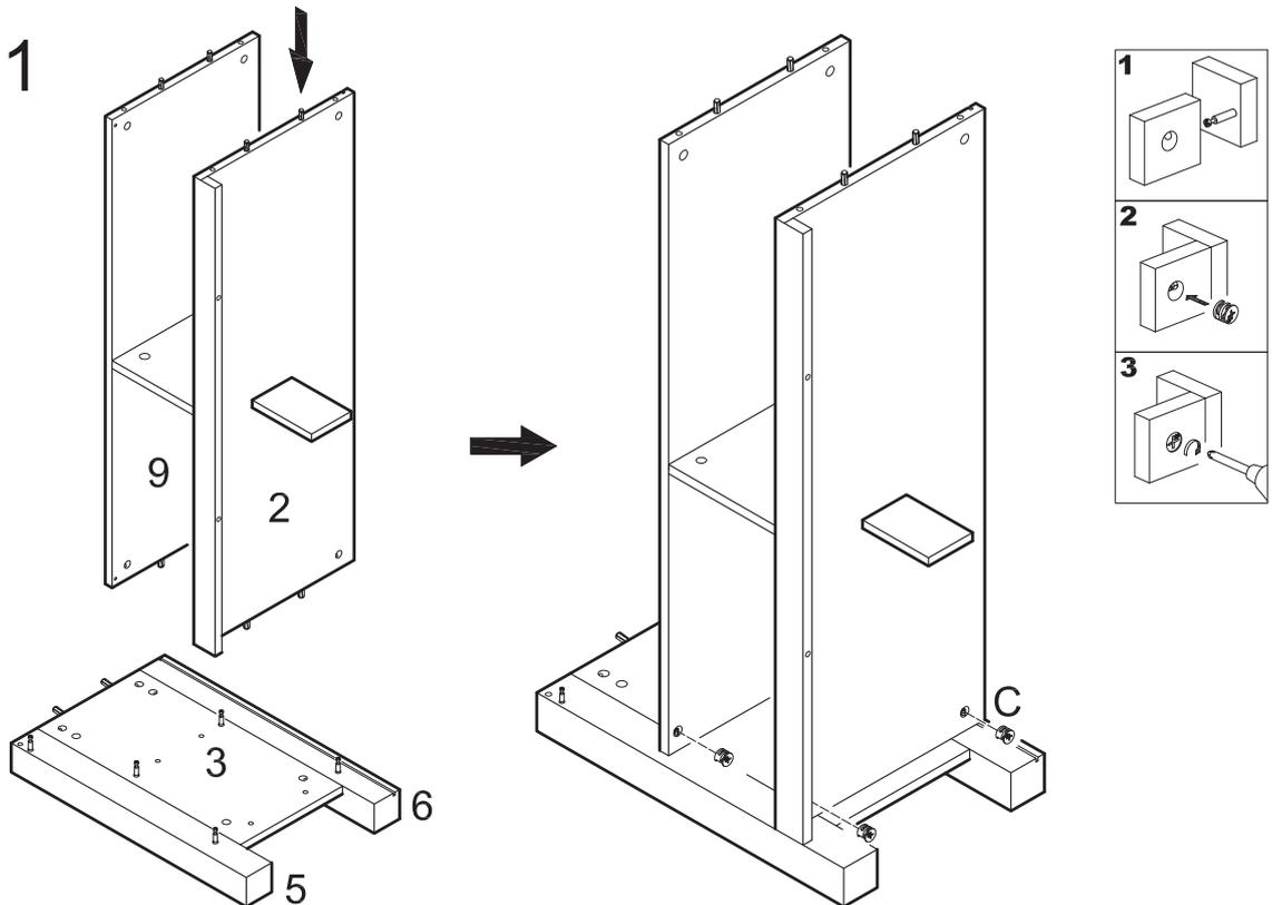
Attach the panel (2,9) assembly to the panel (3) assembly using cam bolts and dowels as guides. Insert cam locks (C) into panel (2) and shelf (9) and tighten with a screwdriver. Two cam locks (C) will be inserted into panel (2) and into shelf (9).
