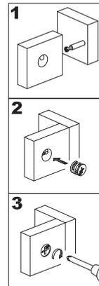
Attach the panel (4) assembly to panel (2), shelf (9) and slat (10) using cam bolts and dowels as guides. Insert cam locks (C) into panel (2), shelf (9) and slat (10) and tighten with a screwdriver.
