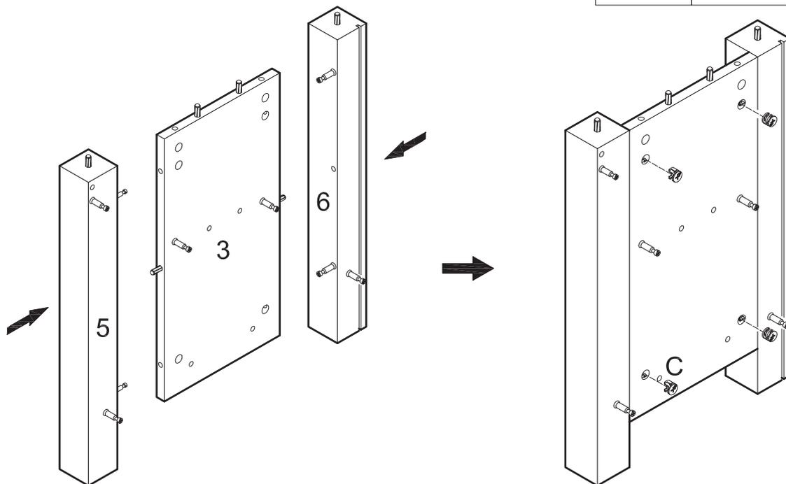
Attach legs (5,6) to panel (3) using cam bolts and dowels as guides. Insert cam locks (C) into panel (3) and tighten with a screwdriver.
