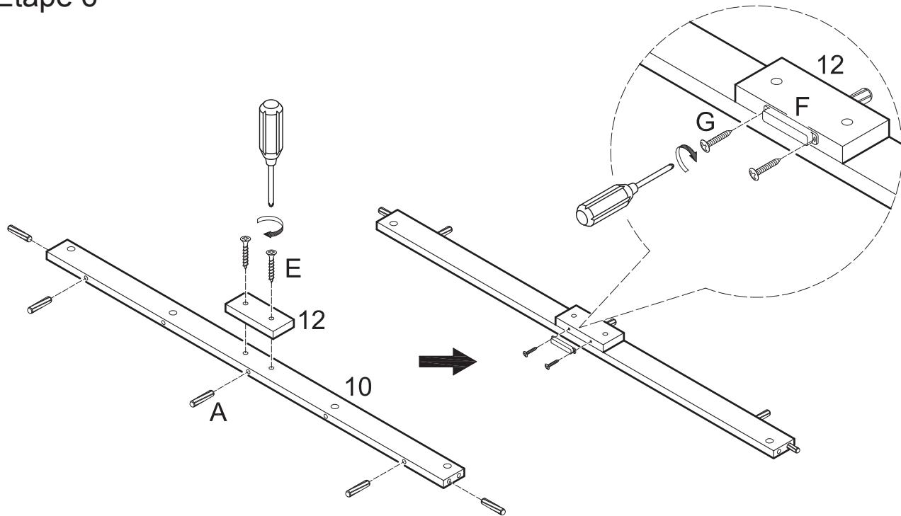
Insert dowels (A) into slat (10). Attach slat (12) to slat (10) using screws (E). Attach door stopper (F) to slat (12) using screws (G).
