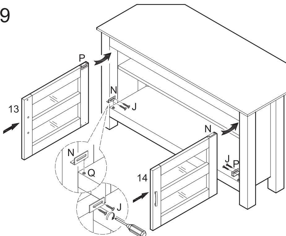
Insert door hinge (N) into bottom left bottom plastic pivot (Q). Slide door (13) into place, inserting flange of door hinge (P) into top left plastic pivot (Q). Secure door hinge (N) to door (13) using screws(J). Insert door hinge (P) into bottom right plastic pivot (Q).Slide door (14) into place,inserting flange of door hinge (N) into top right plastic pivot (Q).Secure door hinge (P) to door (14) using screws (J).
