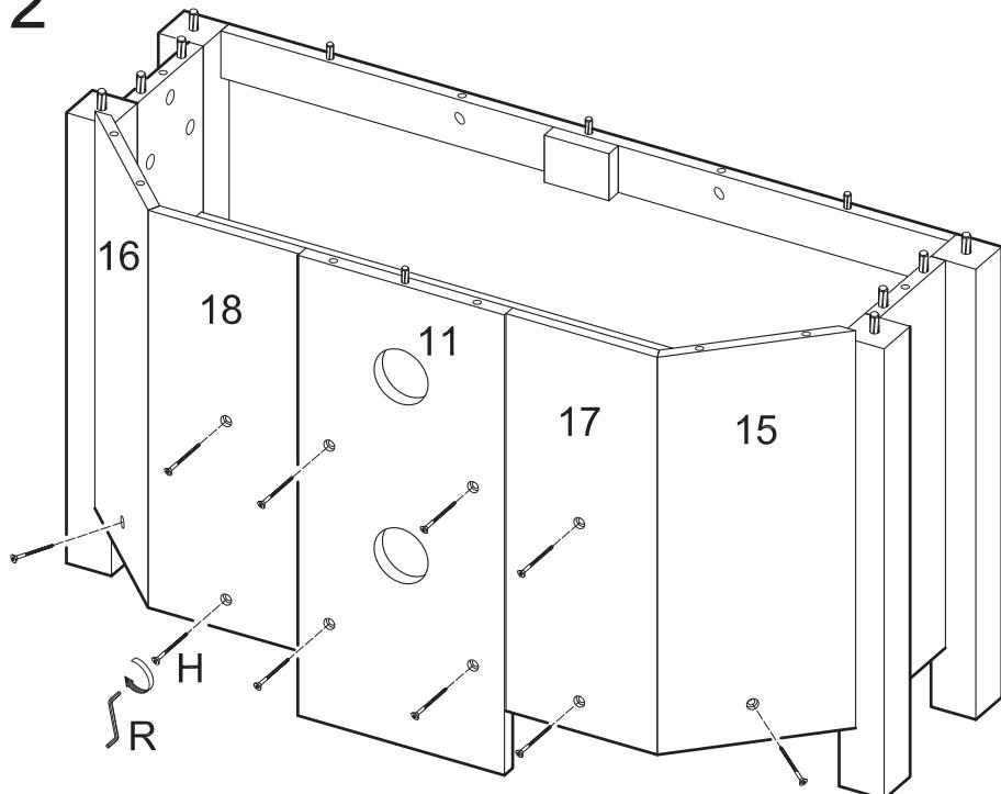
Attach back panels (11,15,16,17,18) to the frame assembly using bolts (H). Tighten bolts (H) with wrench (R). Bolts (H) will screw through back panels (11,15,16,17,18) and into either panel (2) or shelf (9).
