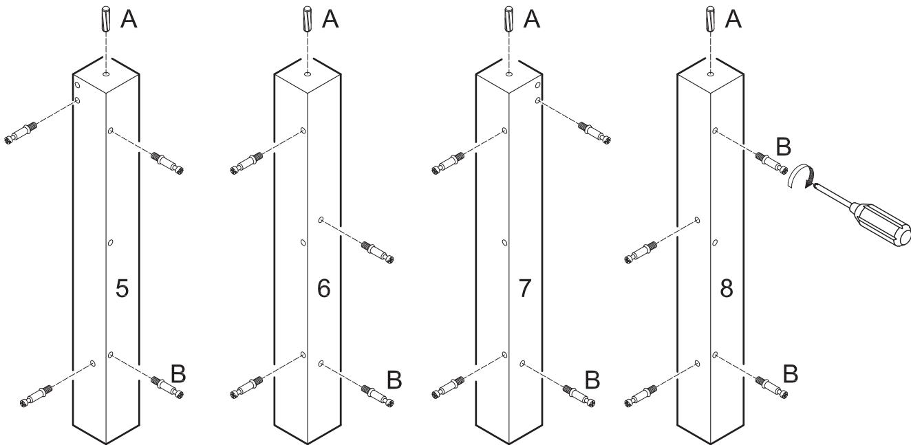
Insert dowels (A) into legs (5,6,7,8). Screw cam bolts (B) into legs (5,6,7,8).
