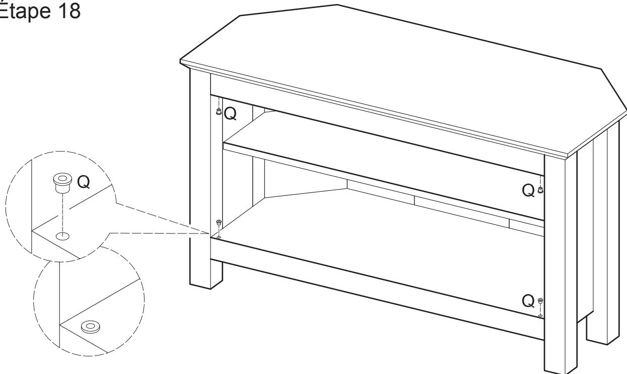
Insert plastic pivots (Q) into panel (2) and slat (10).
