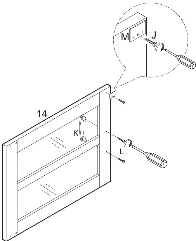
Attach handles (K) to doors (13, 14) using screws (L). Attach door stopper plates (M) to doors (13, 14) using screws (J).
