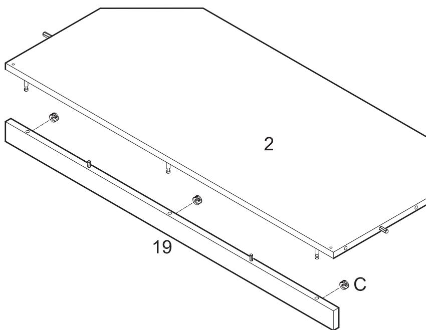
Attach slat (19) to panel (2) using cam bolts and dowels as guides. Insert cam locks (C) into slat (19) and tighten with a screwdriver.
