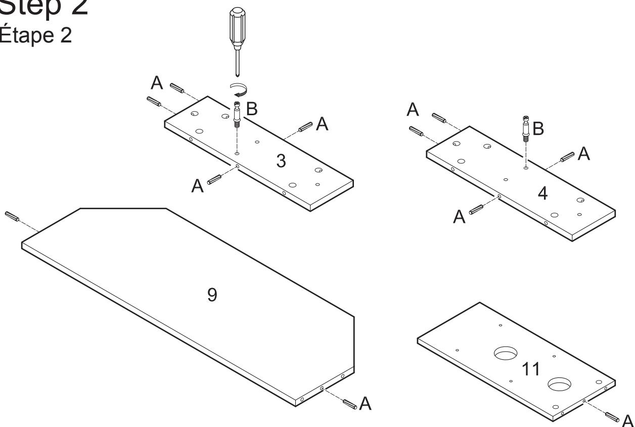
Insert dowels (A) into shelf (9), panels (3,4) and back panel (11). Screw cam bolts (B) into panels (3,4).
