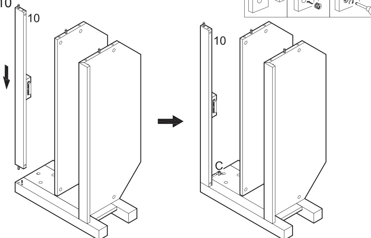
Attach slat (10) to panel (3) using cam bolt and dowel as guides. Insert cam lock (C) into slat (10) and tighten with a screwdriver.
