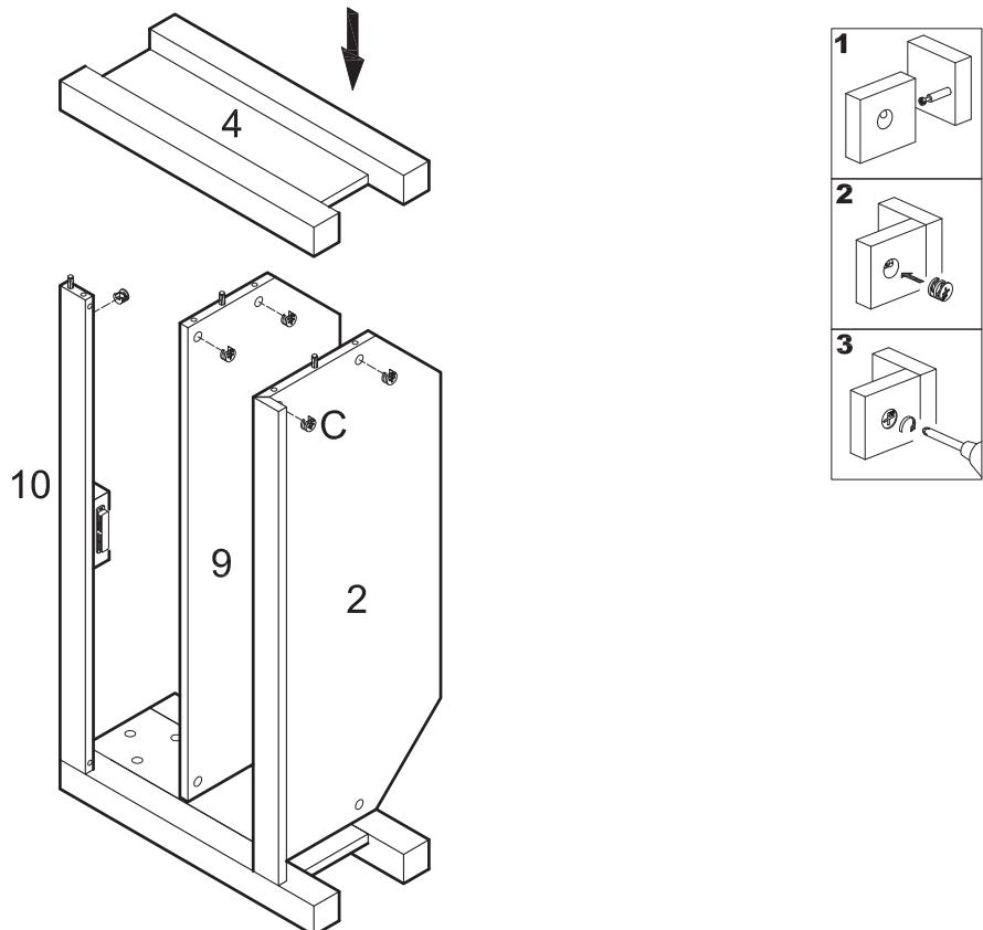
Insert cam locks (C) into panel (2), shelf (9) and slat (10). Attach panel (4) to panel (2), shelf (9) and slat (10) using cam bolts and dowels as guides. Tighten cam locks (C) with a screwdriver.
