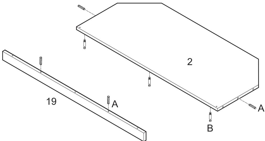
Screw cam bolts (B) into panel (2). Insert dowels (A) into panel (2) and slat (19).
