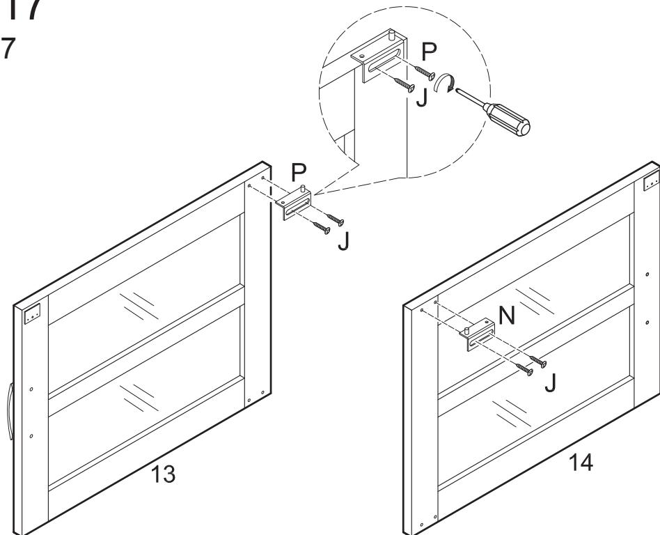
Attach door hinge (P) to door (13) using screws (J). Attach door hinge (N) to door (14) using screws (J).
