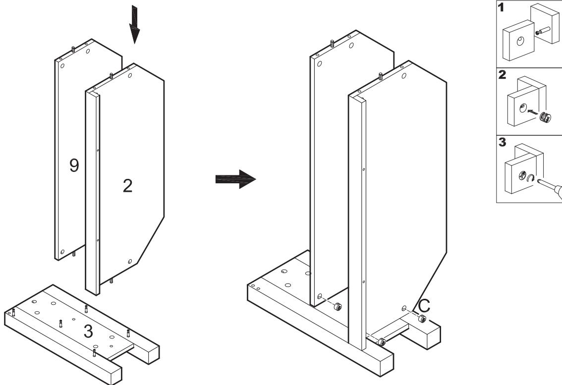
Attach panel (2) and shelf (9) to panel (3) using cam bolts and dowels as guides. Insert cam locks (C) into panel (2) and shelf (9) and tighten with a screwdriver. Two cam locks (C) will be inserted into panel (2) and into shelf (9).
