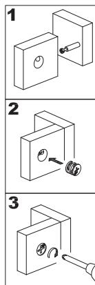
Insert cam locks (C,D) into the frame assembly. Attach stand top (1) to the frame assembly using cam bolts and dowels as guides. Tighten cam locks (C,D) with a screwdriver.
