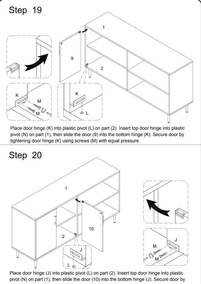
tightening door hinge (J) using screws (M) with equal pressure.
