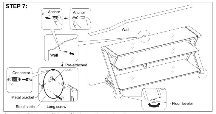
Secure the unit to the wall with the provided tipping restraint hardware kit.
