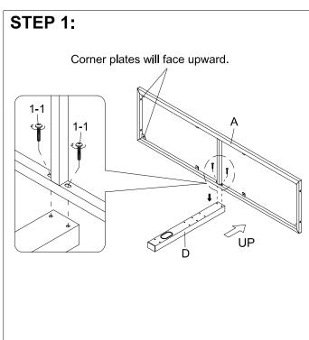
Attach top shelf frame (A) to the spine (D) . Note: Do not over tighten the bolts.
