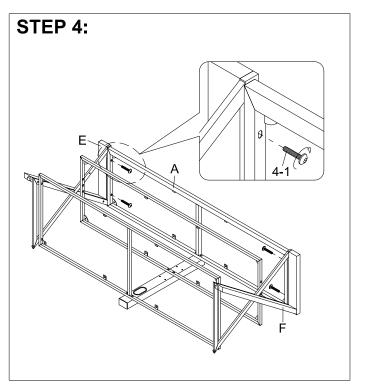
Attach two side frames (E and F) to the top frame (A) . Note: Do not over tighten the bolts.
