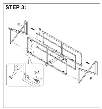
Attach two side frames (E and F) to the middle and bottom shelf frames (B and C).
