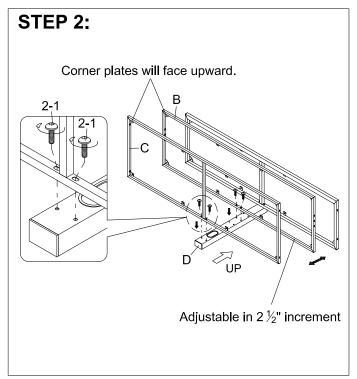
Attach middle and bottom shelf frame (B and C) to the spine (D).
