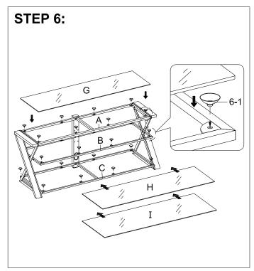
Put the suction cups onto the shelf frames (A, B and C). Place the glass shelves (G, H and I) onto the shelf frames properly.
