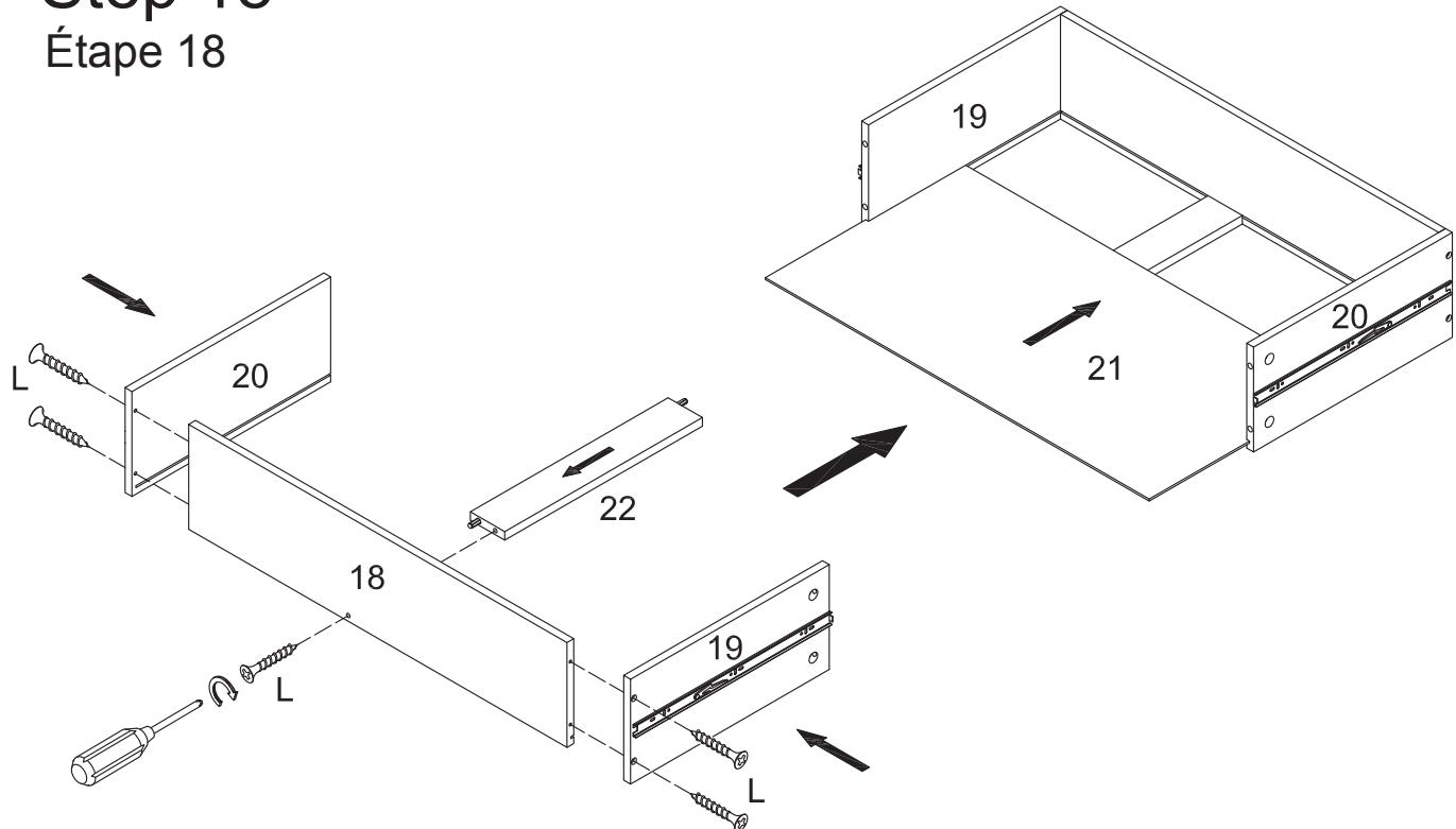
Attach panels (19, 20) to panel (18) using screws (L). Attach support bar (22) to panel (18) using screw (L). Carefully slide panel (21) into the thin grooves as shown in the diagram.
