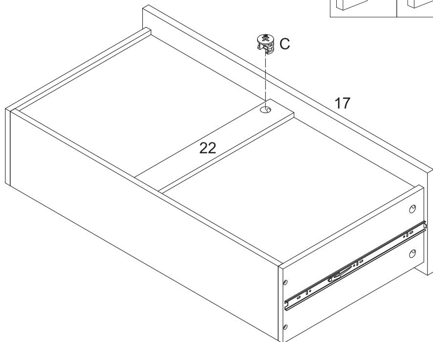
Attach panel (17) to drawer assembly using cam locks (C).
