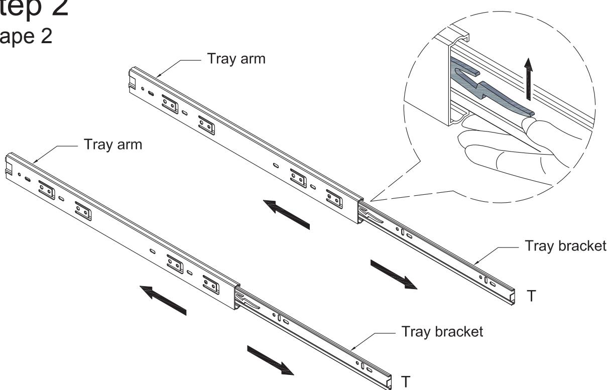
Disassemble keyboard tray slider (T) by sliding the tray arm and tray bracket apart. Depress the small lever of the tray bracket and carefully pull the two pieces apart. Repeat this process for both keyboard tray sliders (T).
