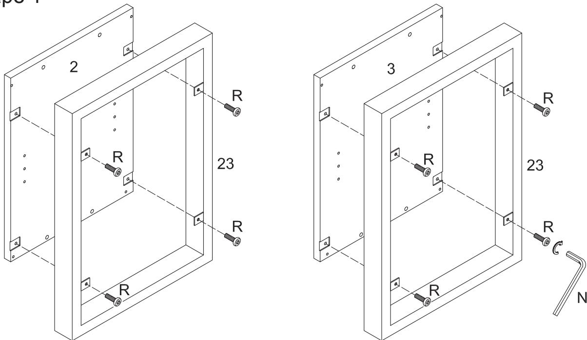
Use wrench (N), bolt (R) to secure the side frame (23) to the side panel (2,3).
