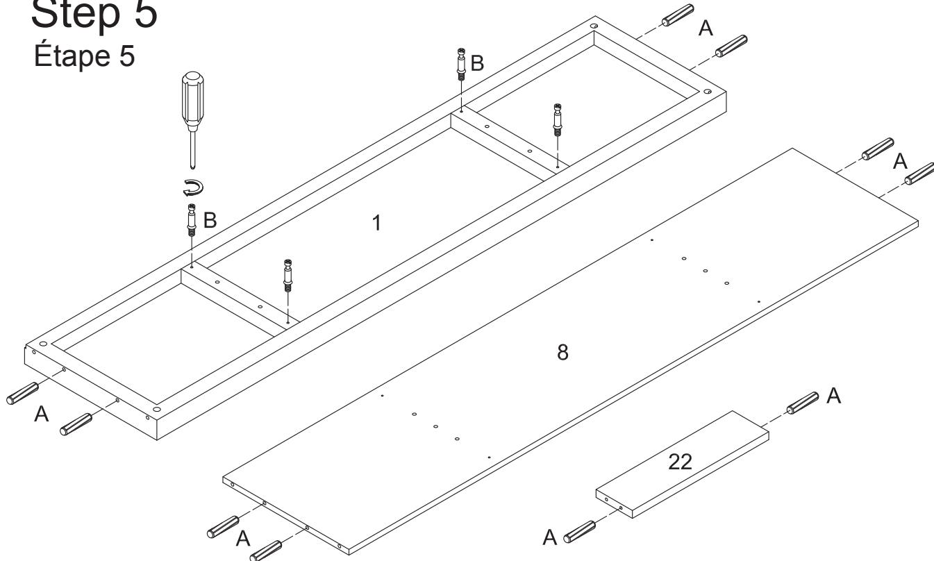
Secure cam bolts (B) into top panel (1). Insert wooden dowels (A) into bottom panels (1,8,22).
