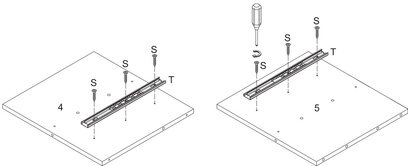
Secure screw (S) to the tray arm of keyboard tray slider (T) to the middle side panel (4,5).
