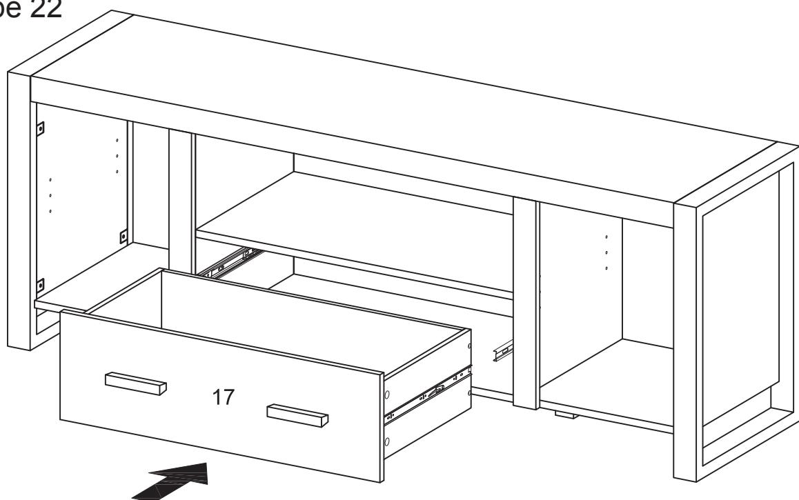
Carefully insert drawer assembly into assembled unit.
