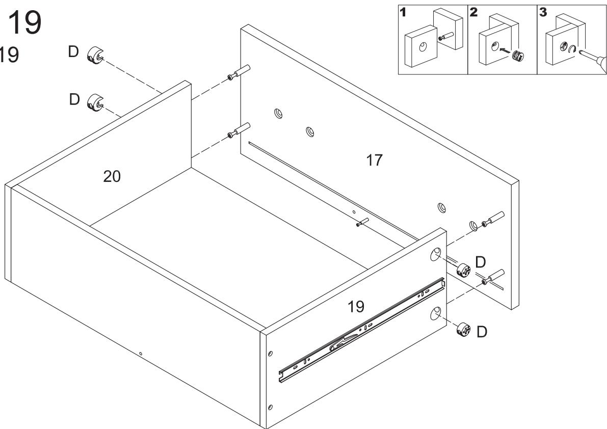
Attach panel (17) to drawer assembly using cam locks (D).
