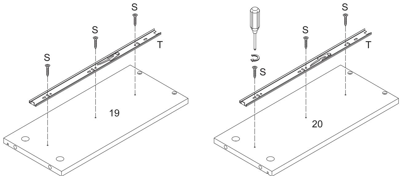
Secure screw (S) to the tray bracket of keyboard tray slider (T) to the drawer side panel (19,20).
