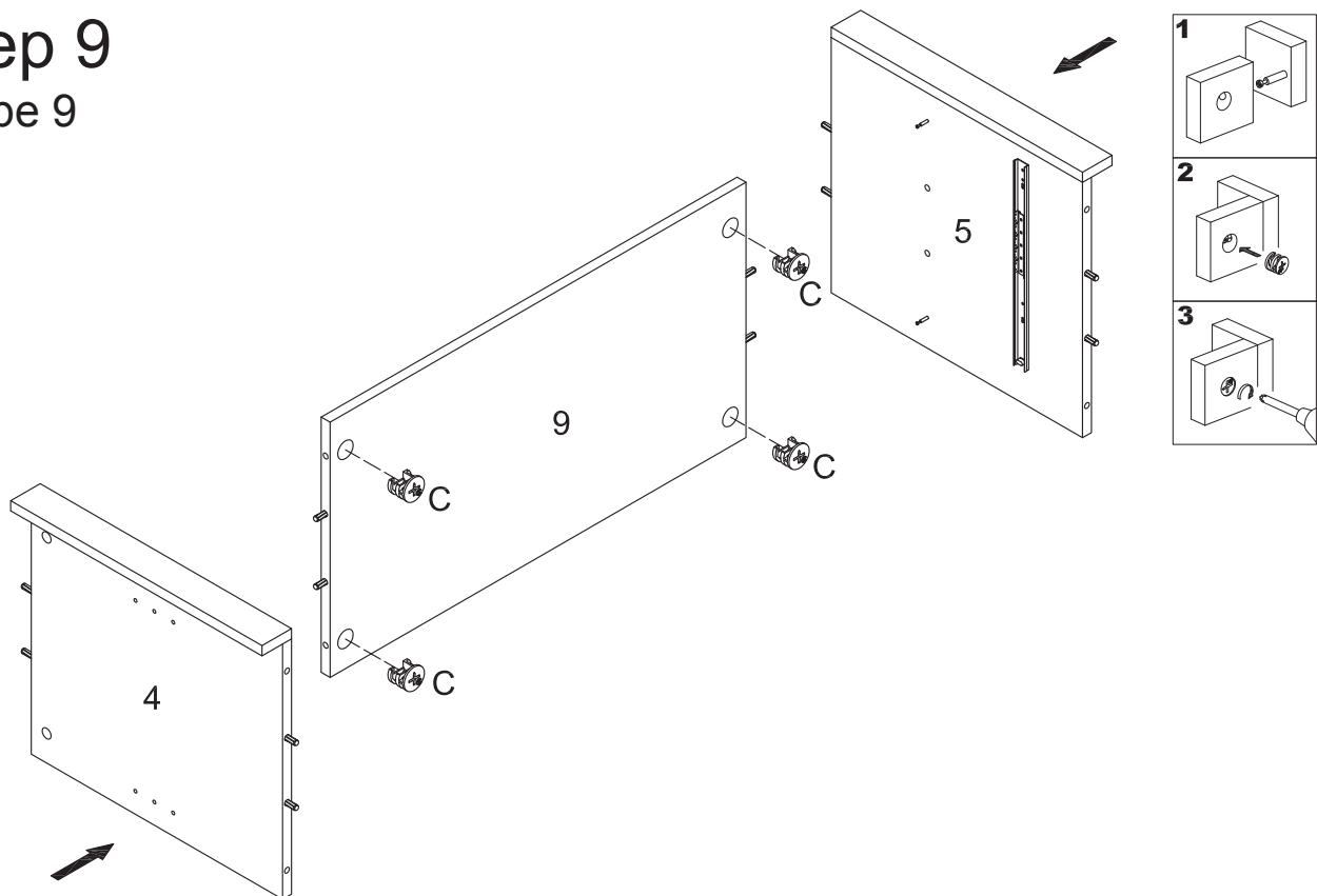
Attach side panels (4, 5) to shelf panel (9) using cam locks (C).
