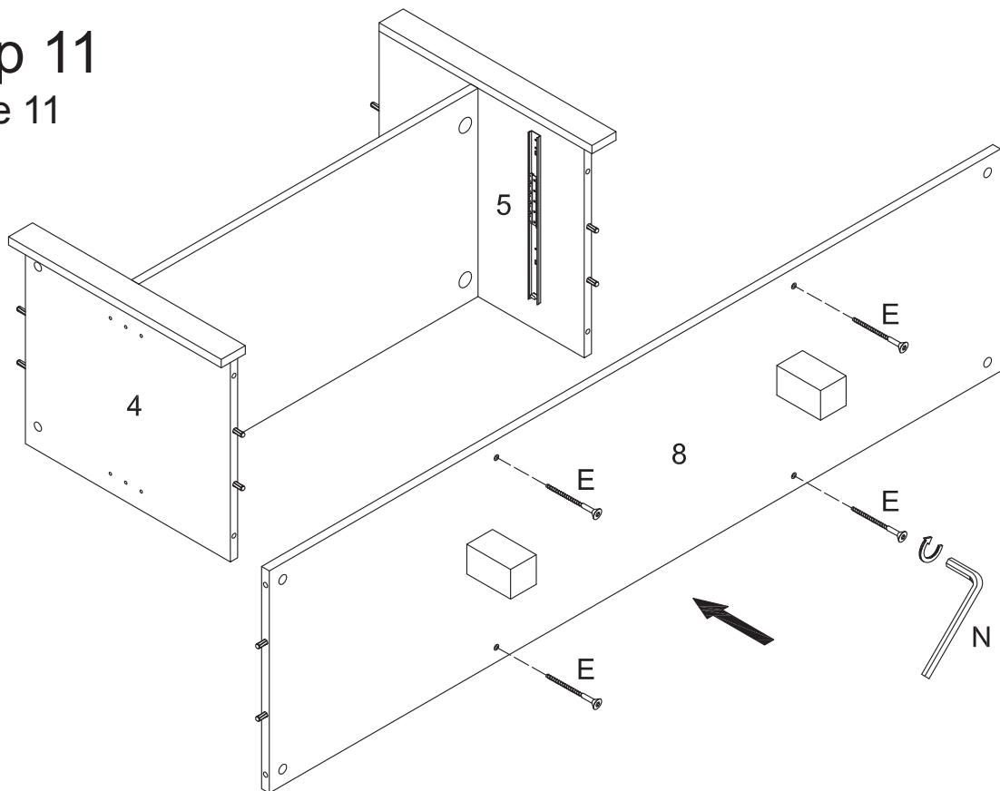
Attach side panels (4,5) to bottom panel (8) using screws (E).
