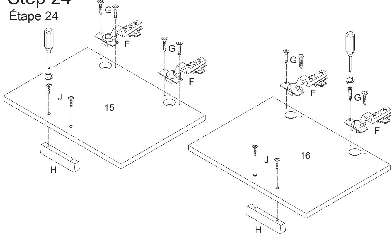
Attach hinge (F) to doors (15, 16) using screws (G). Attach handles (H) using bolts (J).
