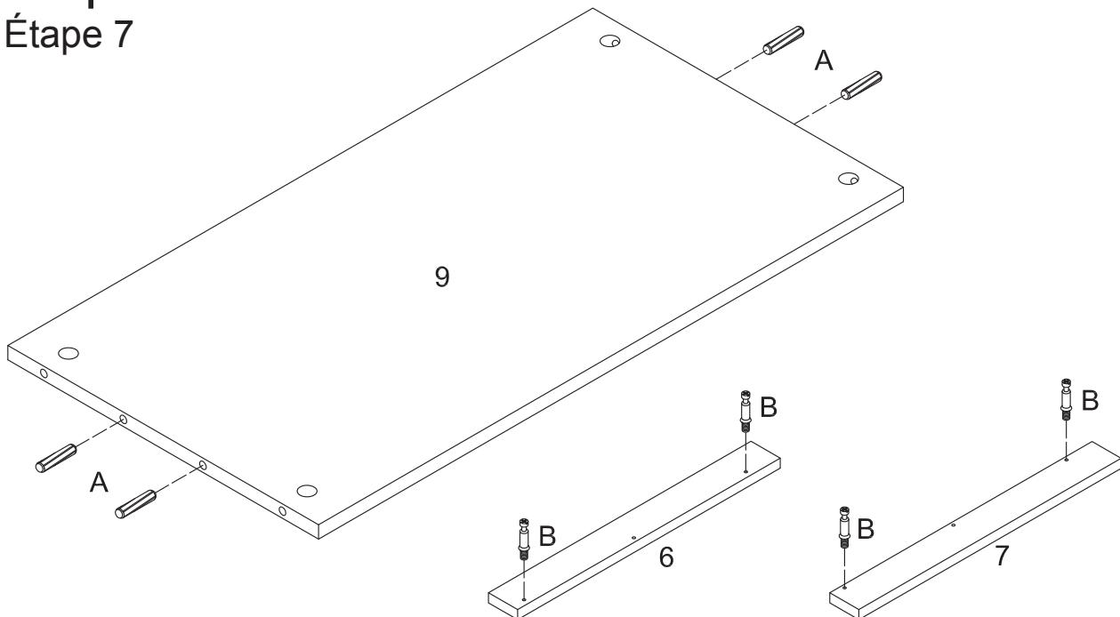
Insert wooden dowels (A) into panel (9). Secure cam bolts (B) into panels (6, 7).
