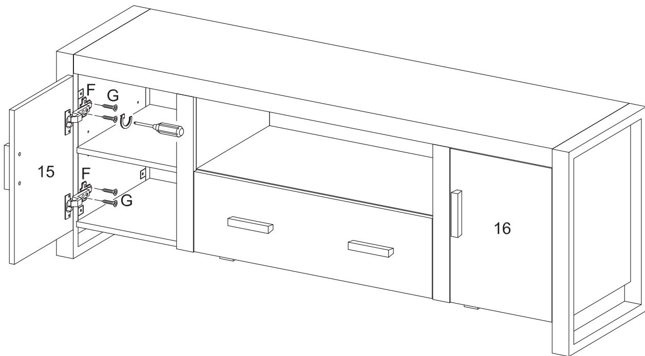
Assemble the doors (15, 16) movable together using screws (G).
