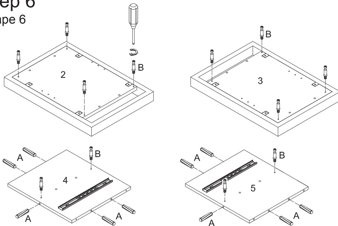
Secure cam bolts (B) into side panels (2, 3, 4, 5). Insert wooden dowels (A) into side panels (4,5).
