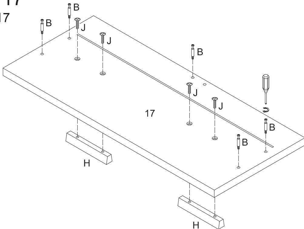
Secure cam bolts (B), attach handles (H) to panel (17) using bolts (J).
