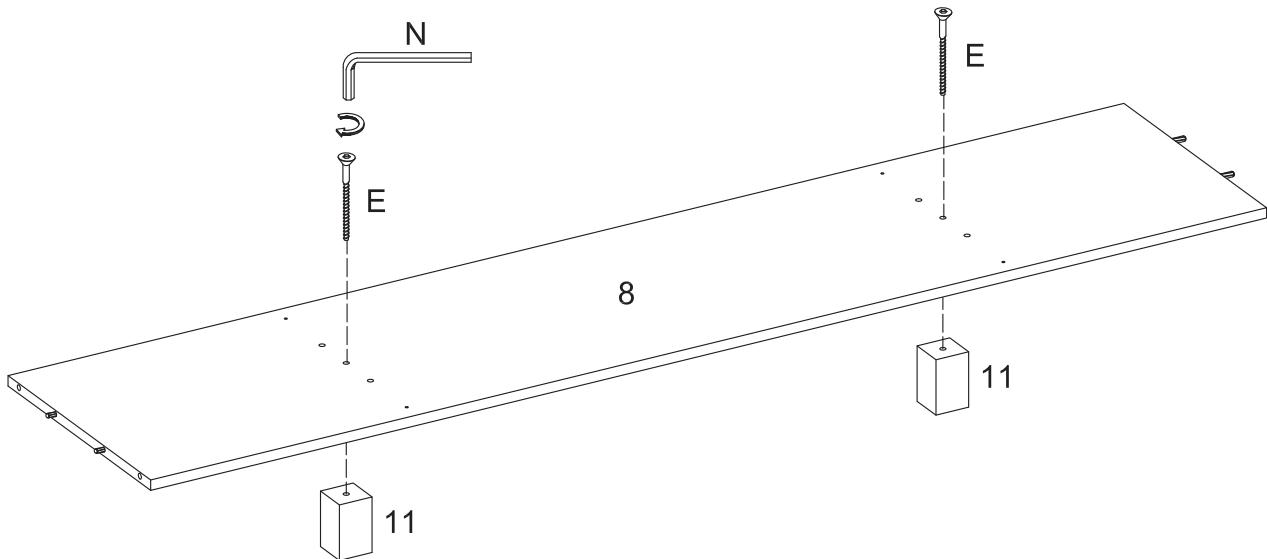
Secure legs (11) to bottom panel (8) using screws (E).
