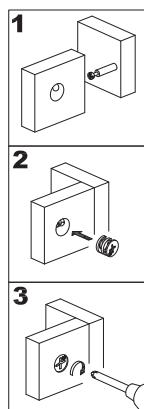
Attach top panel (1) to side panels (4,5) using cam locks (C).
