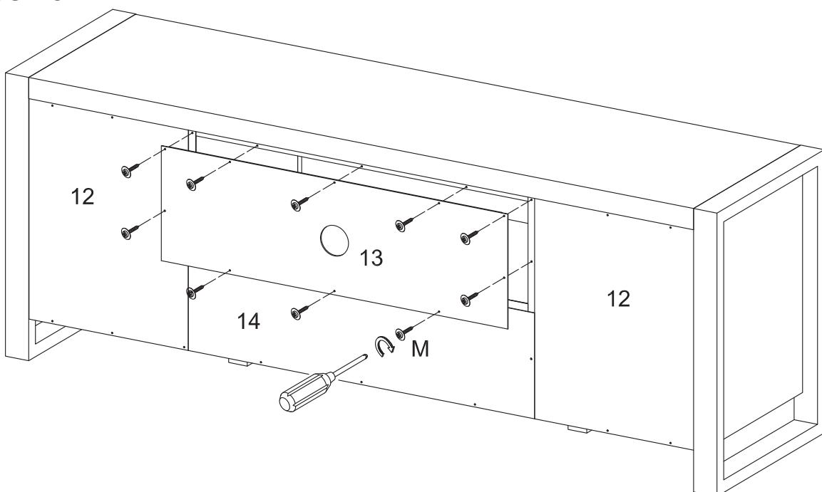
Secure back panel (13) using screws (M).
