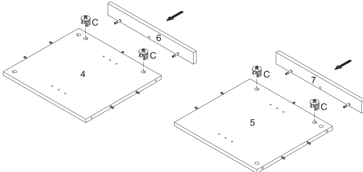
Attach panel (6) to panel (4) using cam locks (C). Attach panel (7) to panel (5) using cam locks (C).
