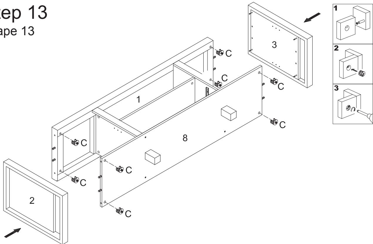
Attach side panels (2,3) to assembled unit using cam locks (C).
