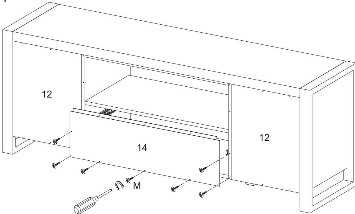
Secure back panel (14) using screws (M).
