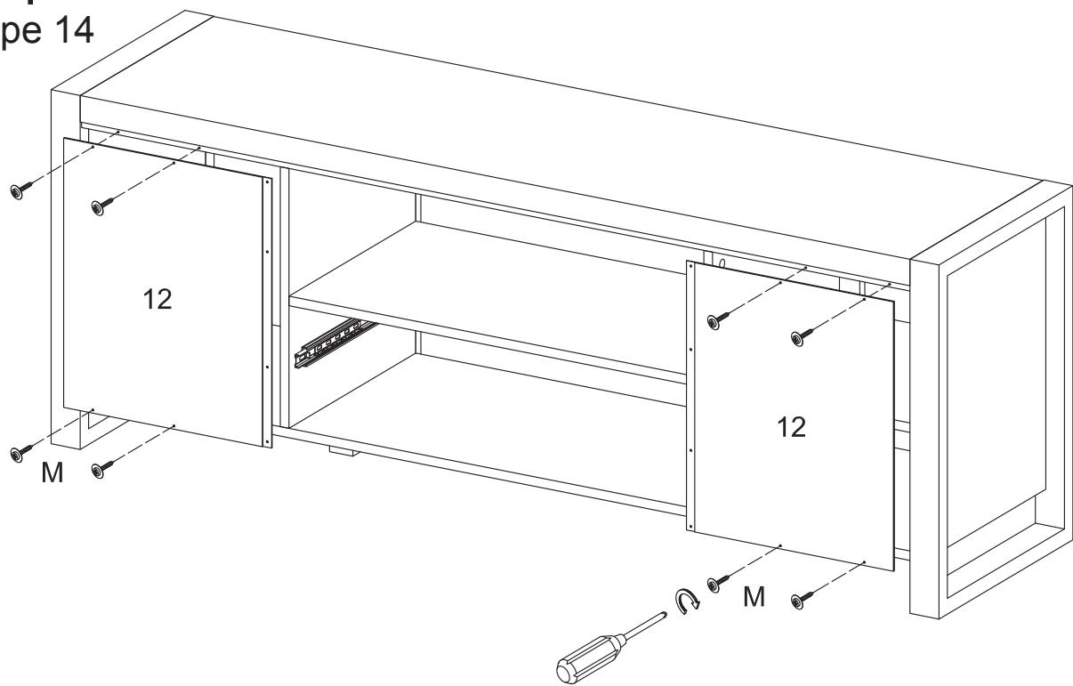
Secure back panels (12) using screws (M).
