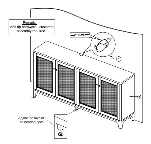
Hardware Pack Location: Anti-tip kit attached in the back panel KD leg inside cabinet
